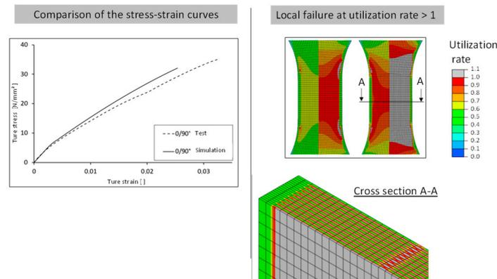
Figure 18. Comparison of deformation behavior and local failure.
