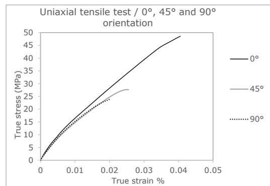
**Figure 1.** True stress-strain curves with different strand orientations ( $0^\circ$ ,  $45^\circ$  and  $90^\circ$ ) [36].
