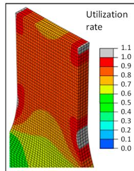
Figure 4. Local failure of the isotropic FEM model.
