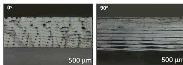
**Figure 3.** Porosity of tensile test rods in the  $0^\circ$  and  $90^\circ$  deflection direction.
