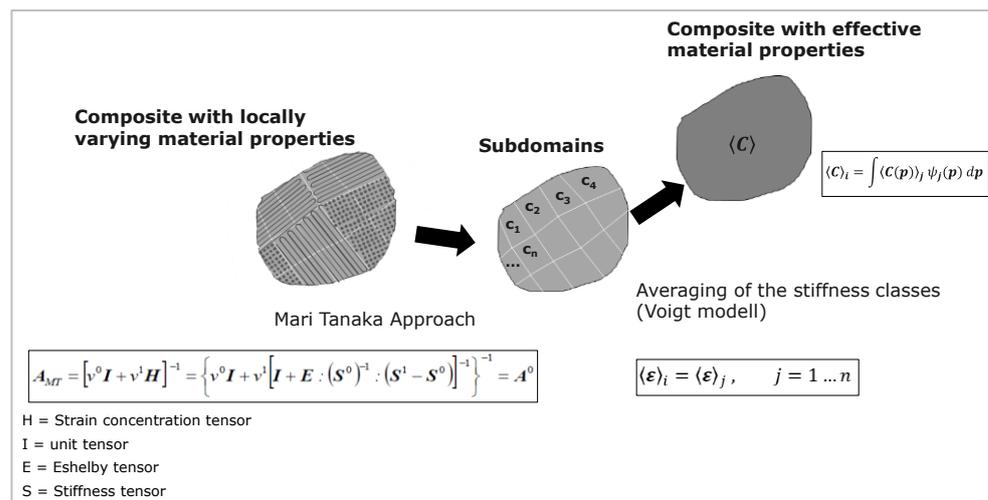
Figure 9. Two-Step Homogenization Scheme.
