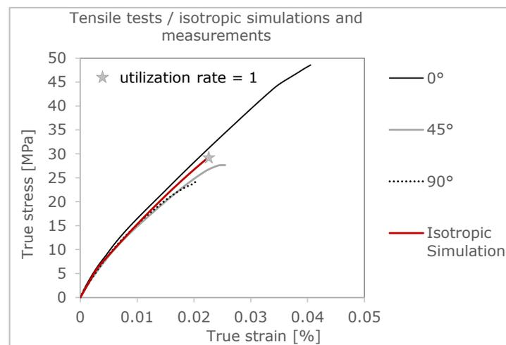
**Figure 5.** Deformation behavior of the isotropic FEM model.
