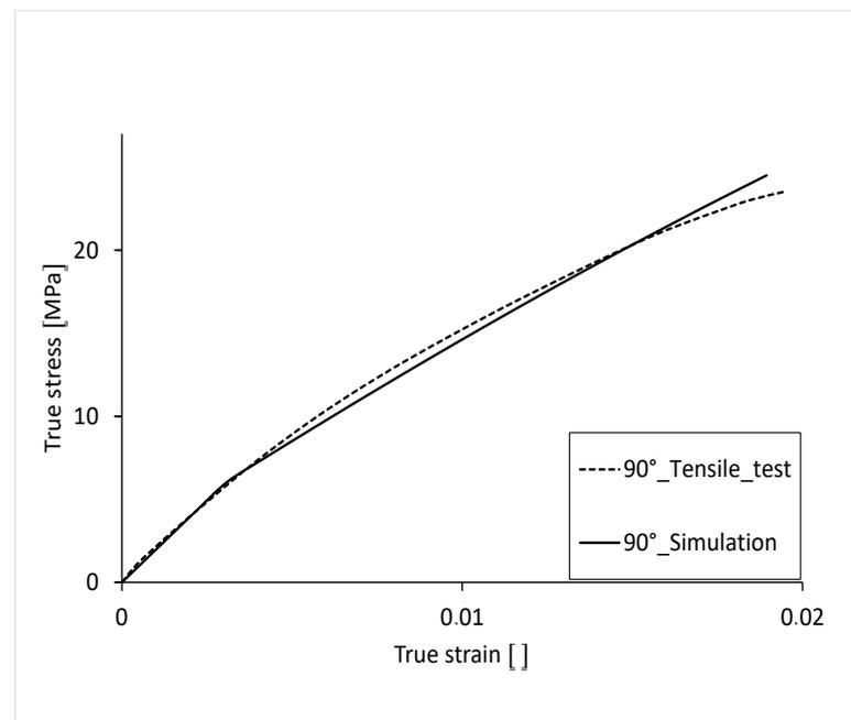
**Figure 16.** Comparison of true stress-strain curve 90°.
