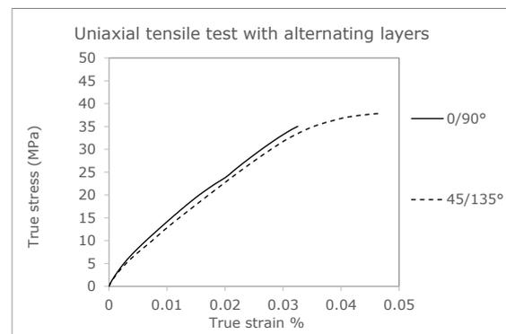
**Figure 2.** True stress-strain curves with cross-layered structured  $0^\circ/90^\circ$  and  $45^\circ/135^\circ$  [36].
