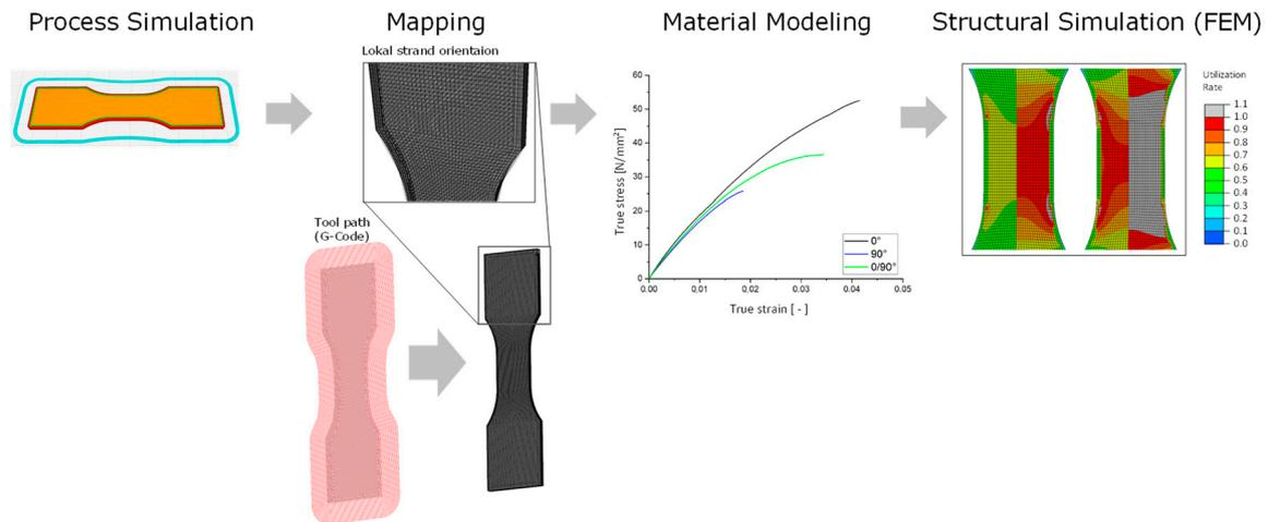
**Figure 6.** Steps of a process and structured coupled simulation considering local manufacturing direction.
