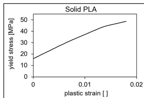
**Figure 10.** Plastic strain–true stress curve for pure PLA.
