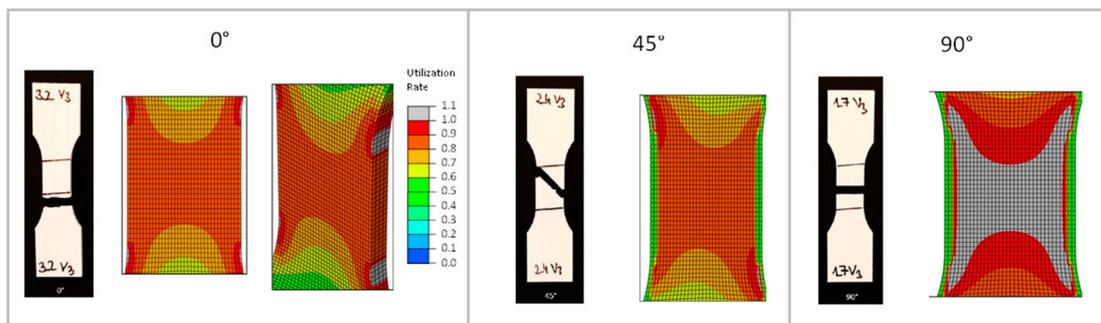
Figure 19. Comparison of the fracture behavior of the tension specimens and simulation.
