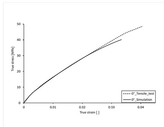
**Figure 12.** Comparison of true stress-strain curve  $0^\circ$ .
