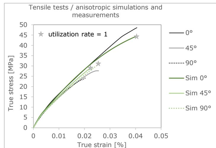
**Figure 11.** Comparison of the true stress-strain curves of tensile test and simulation.
