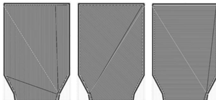
**Figure 7.** Top view of strand orientation in slicing software: 0°, 45°, and 90°.
