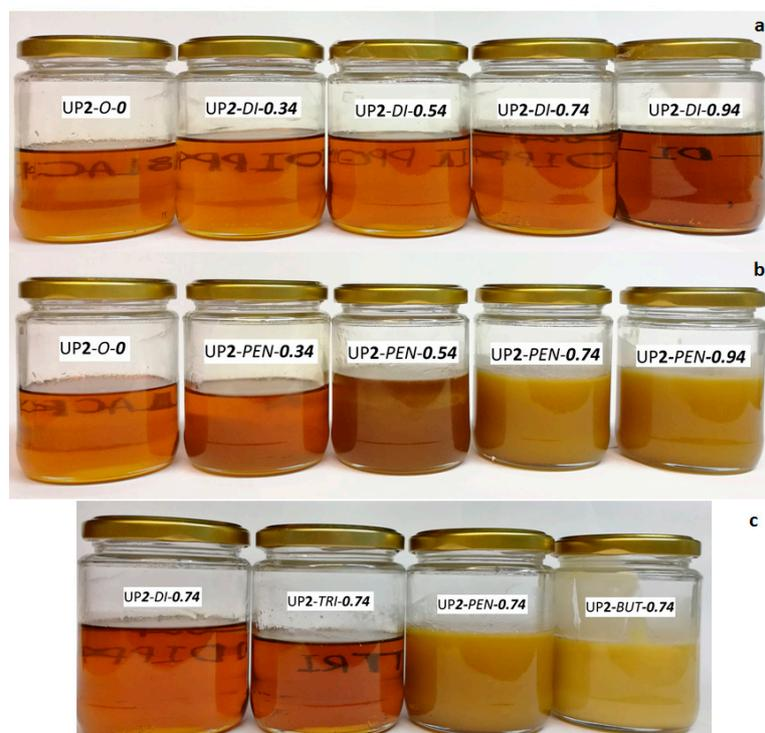
**Figure 9.** The appearance of samples made in two-stage processing: (a) di-PPG chain extended samples compared with the blank sample UP1-O-0; (b) pentanediol chain extended samples compared with the blank sample UP1-O-0; (c) samples with a 0.74 molar ratio of different chain extenders.
