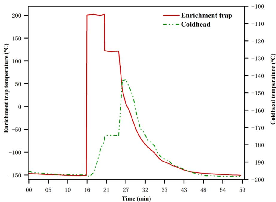
**Figure 3.** Cooling and heating cycles of the sampling enrichment trap and coldhead of the cooler loops.
