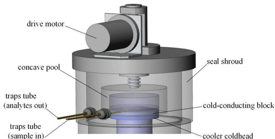
**Figure 2.** Technical drawing of the coldhead and cryotrap placed inside.
