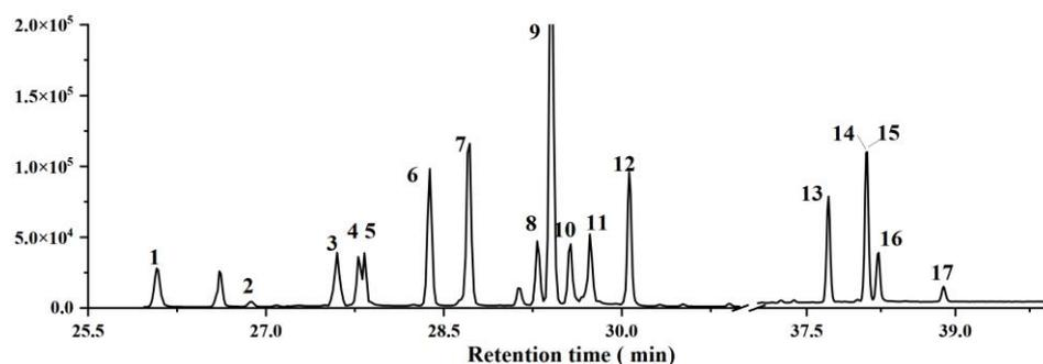
**Figure 5.** Separation of BVOCs using a DB-624 column. VOC mixing ratios were approximately 2 ppbv. The peaks in order from left to right were: 1.  $\alpha$ -Pinene, 2. Camphene, 3. Sabinene, 4.  $\beta$ -Myrcene, 5.  $\beta$ -Pinene, 6. 2-Carene, 7. 3-Carene, 8. D-limonene, 9. p-Cymene, 10. Ocimene, 11. Cineole, 12.  $\gamma$ -Terpinene, 13. Isolongifolene, 14. Longifolene, 15.  $\alpha$ -Cedrene, 16.  $\beta$ -Caryophyllene, 17.  $\alpha$ -Caryophyllene.
