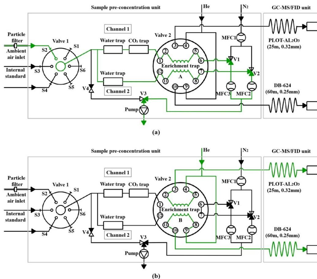
**Figure 1.** Flow scheme showing the gas flow. (a) Position A in Valve 2, sampling pre-concentration state; (b) Position B in Valve 2, sampling injection state. The green line shows the gas path. S1–S6 denote the positions of Valve 1. The number of Valve 2 denote the Valve positions. V1, V2, V3, V4 denote solenoid valves.
