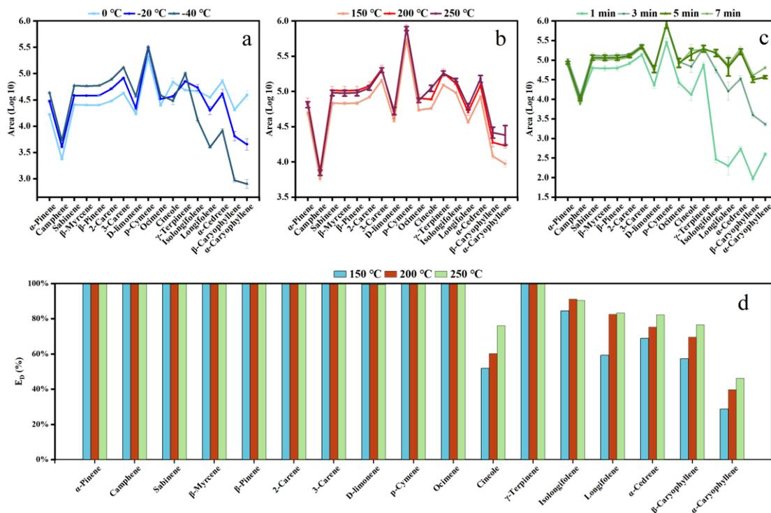
**Figure 4.** Optimization of pre-concentration unit conditions for BVOC measurements. (a) the water trap temperature, (b) the desorption temperature, (c) the desorption time, (d) the desorption efficiency. The error bars represent reproducibility ( $n = 3$ ).
