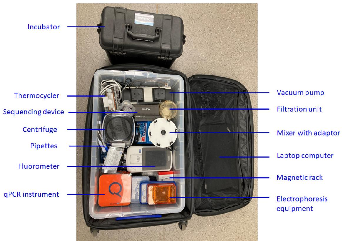
**Figure 4.** Portable laboratory for comprehensive water microbiology by next generation sequencing (NGS), quantitative polymerase chain reaction (qPCR), and culturing. Adapted from [27,124].
