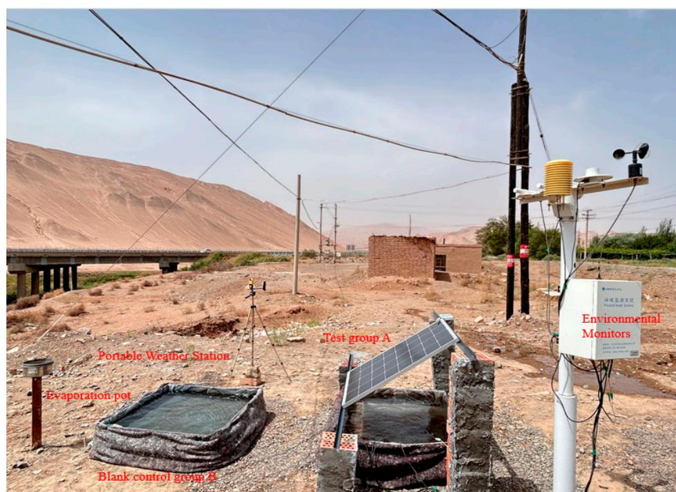
**Figure 4.** Water-based piled PV test diagram.
