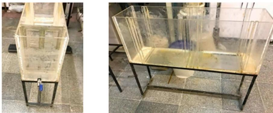
**Figure 2.** The plexiglass with dimensions of  $0.25 \times 0.40 \times 1 \text{ m}^3$  was used as the pulp storage pond.
