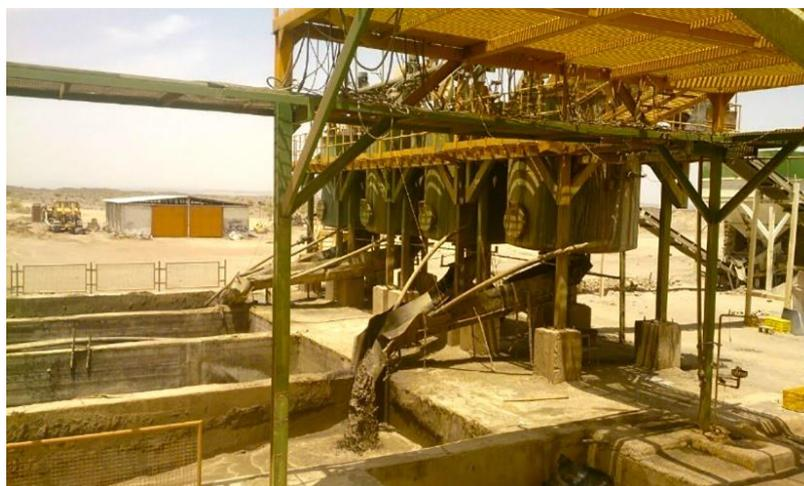
**Figure 1.** Arrangement of the tanks for mixing pulps and draining to the ponds with a gradient of 5% at Nasim mine. The tank's length and diameter were 3 and 3.5 m, respectively.
