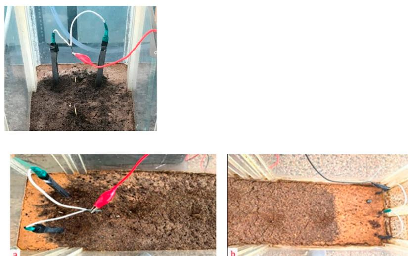
**Figure 7.** The electrodes were placed vertically in the soil to apply the electrokinetic process: (a) anodes and (b) cathodes.
