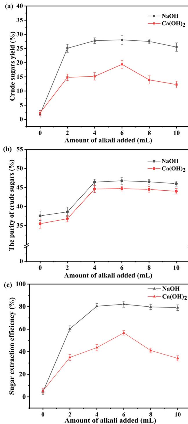
**Figure 1.** Effect of alkali addition on (a) sugar yield; (b) purity; (c) sugar extraction efficiency. Alkali digestion time: 45 min.
