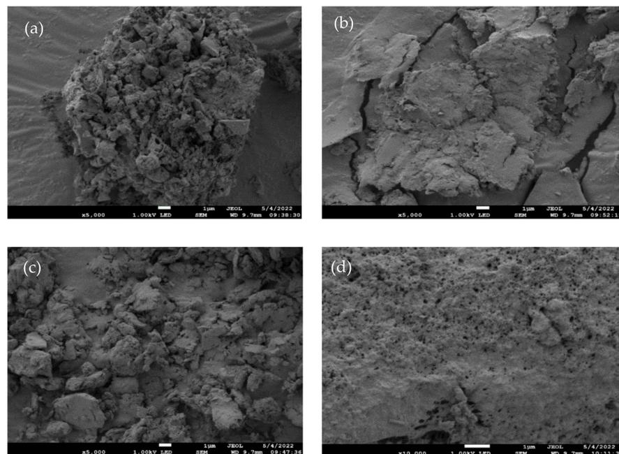
**Figure 6.** The SEM images:(a) raw SS; (b) thermal–alkali, for 60 min; (c) thermal–alkali and ultrasound, 20 min; (d) extracted sugars under the condition of the 6 mL NaOH addition, digestion time 60 min, and 20 min ultrasound time.
