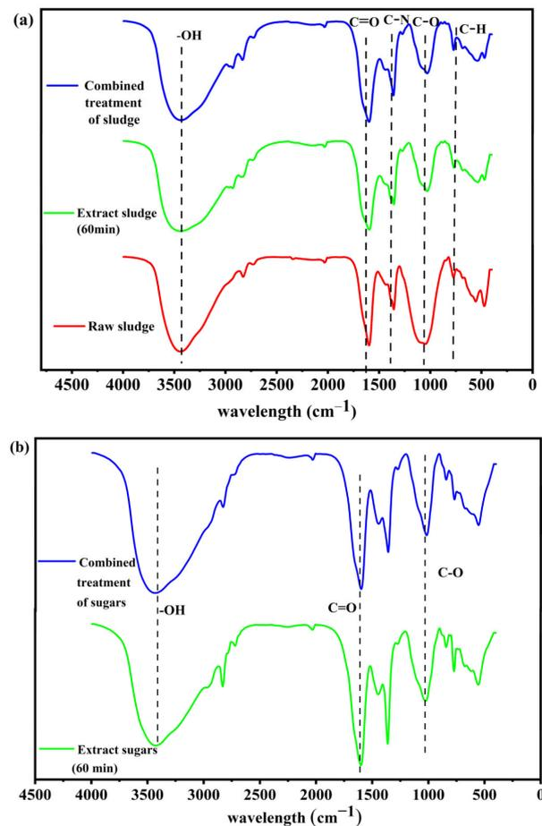
**Figure 7.** The FTIR spectra of (a) raw sludge and treated sludge residue; (b) extracted sugars.
