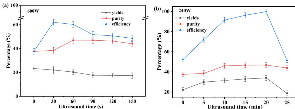
**Figure 3.** Effect of ultrasound power and time on the efficiency of sugar extraction: (a) 600 W; (b) 240 W. All experiments were performed after the addition of 6 mL of NaOH solution. Extraction time: 60 min.
