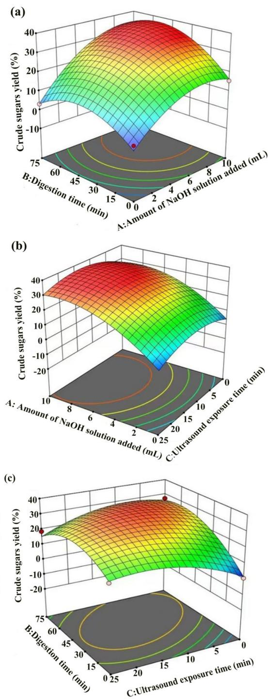
**Figure 5.** Response surface plots of crude sugar yield: (a) NaOH solution added and digestion time; (b) NaOH solution added and ultrasound exposure time; (c) ultrasound exposure time and digestion time.
