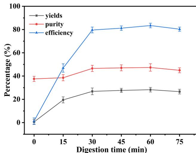
**Figure 2.** Effects of digestion time on sugar extraction under the 6 mL NaOH addition.
