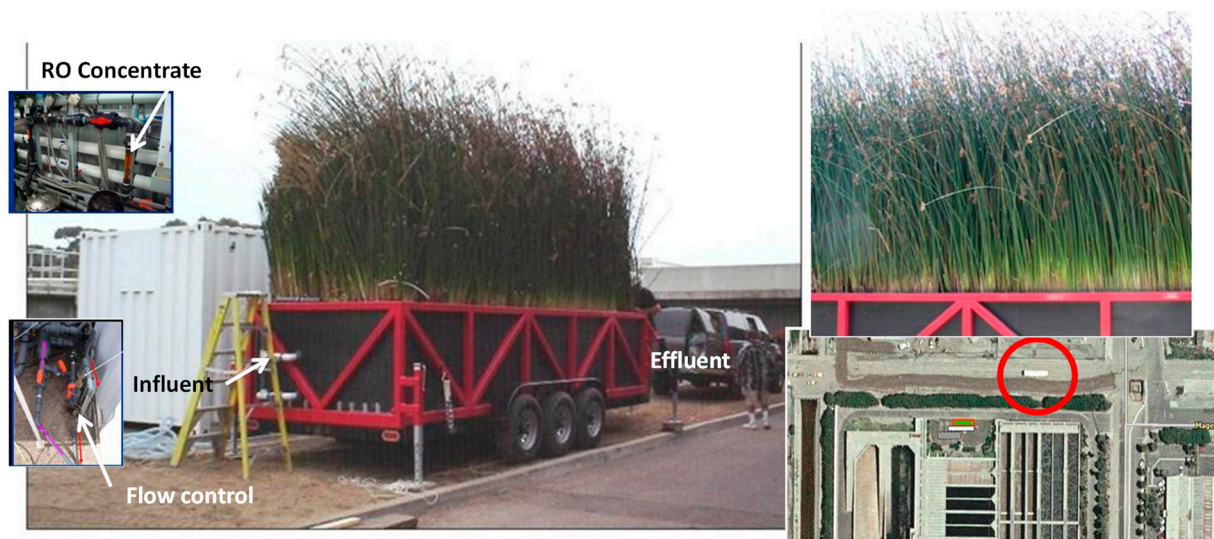
Figure 7. The MES wetland system for Pilot Study 2. The white trailer on the left is the AWPF pilot system and the wetland trailer is equipped with a solar cell to operate the pump used for water circulation. The right top photo shows lively bulrush plants after the 9-month-long pilot study with intense ROC pollution and the bottom photo shows the pilot study layout plan at the AWPF. The red circle shows the pilot plant at the AWPF.
