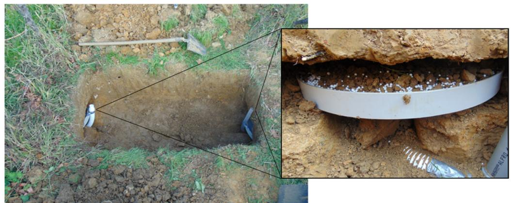
**Figure 4.** Setting up of the zero tension lysimeters (50 cm in diameter) at the hilltop and the footslope at a 40 cm depth.
