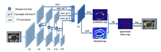
**Figure 2.** Structure of DBNet—DBNet is a novel network architecture for real-time scene text detection with differentiable binarization.
