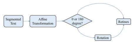
**Figure 5.** The flow chart of text direction classification.
