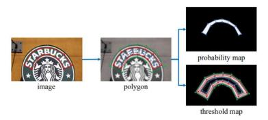
**Figure 4.** Example result of label generation for circular symmetric shape containing text. The annotation of the text polygon is visualized in red lines. The shrunk and dilated polygon are displayed in blue and green lines, respectively [3].
