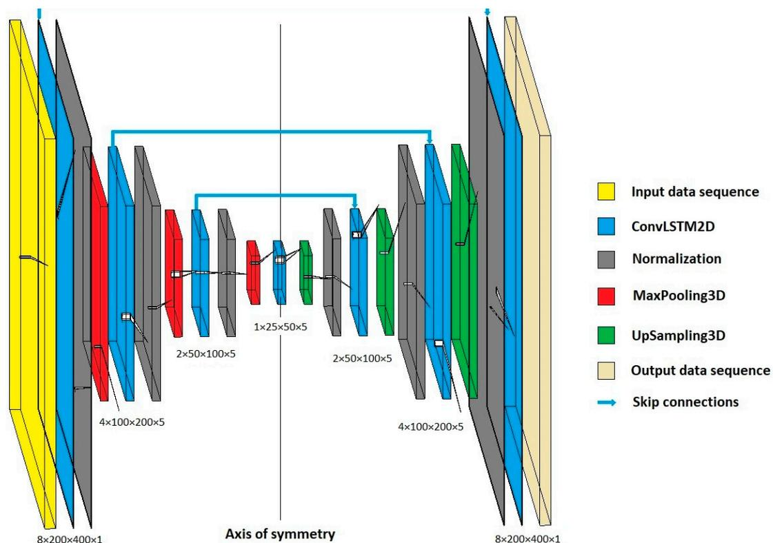
**Figure 1.** Proposed structure of the symmetric U-Net architecture.
