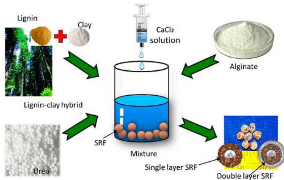
**Figure 3.** The synthesis procedure of double-layer SRFs using bio-based coating materials (reproduced from ref. [59]; copyright 2020 American Chemical Society).
