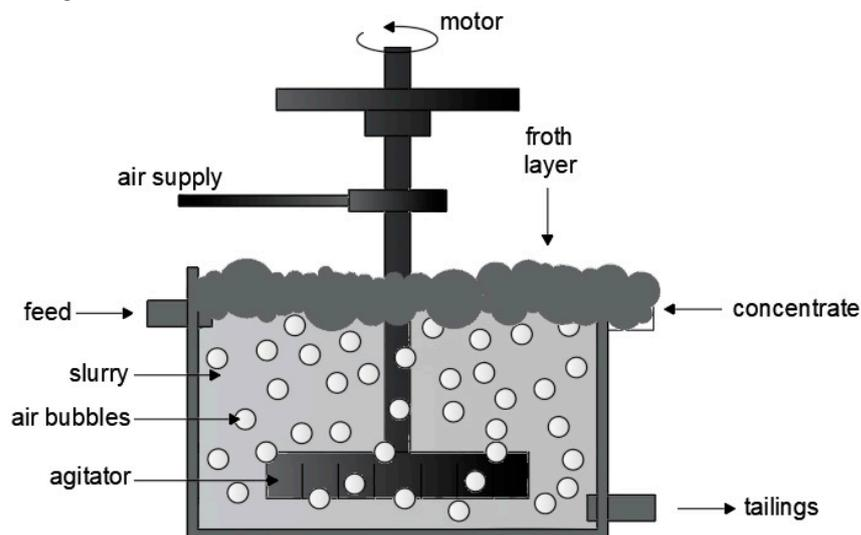
**Figure 1.** Flotation cell.
