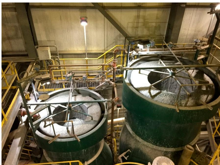
**Figure 2.** Photo of real flotation cells from the processing plant (photo taken by the authors).
