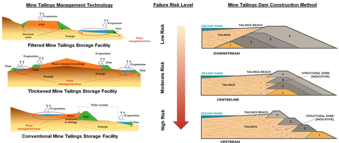
**Figure 1.** Mine tailings management technologies, mine tailings dam construction methods, and associated failure risk levels [19].
