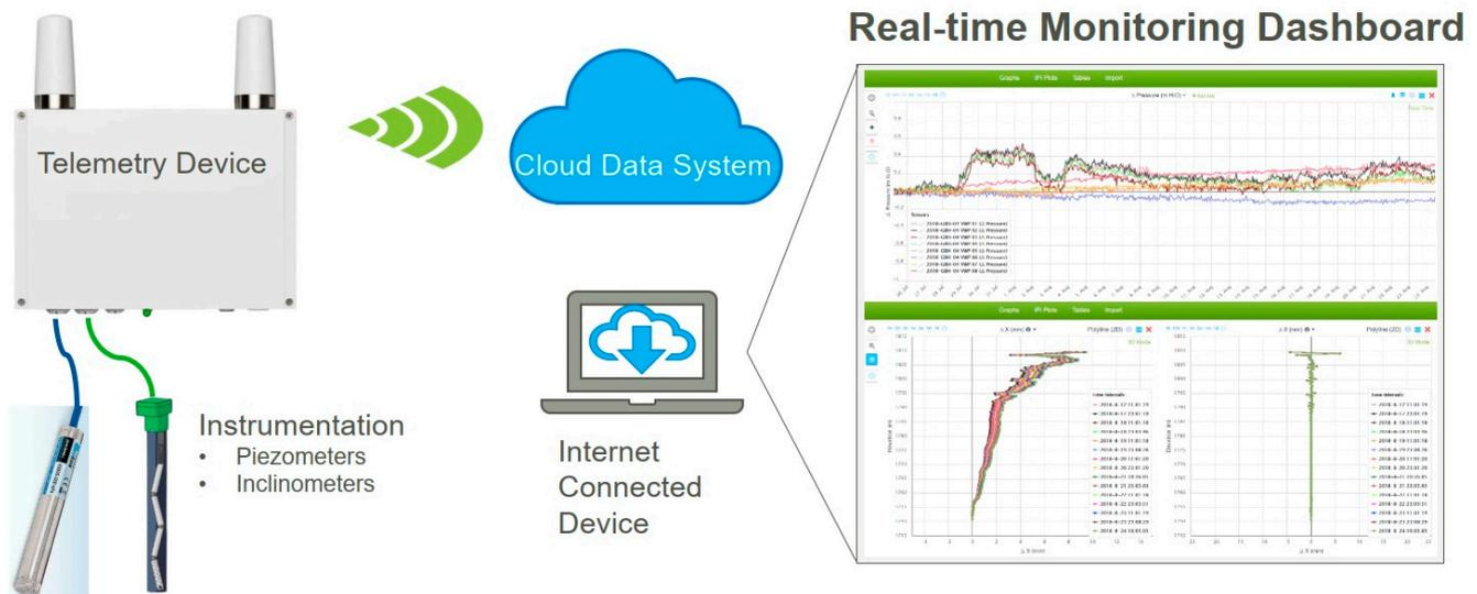
**Figure 24.** An example of the implementation of telemetry technology in mine TSF monitoring.
