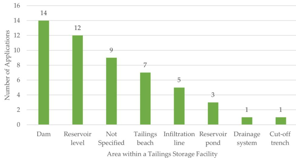
Figure 19. Areas within a TSF where sensors are used to monitor structural health and safety management.
