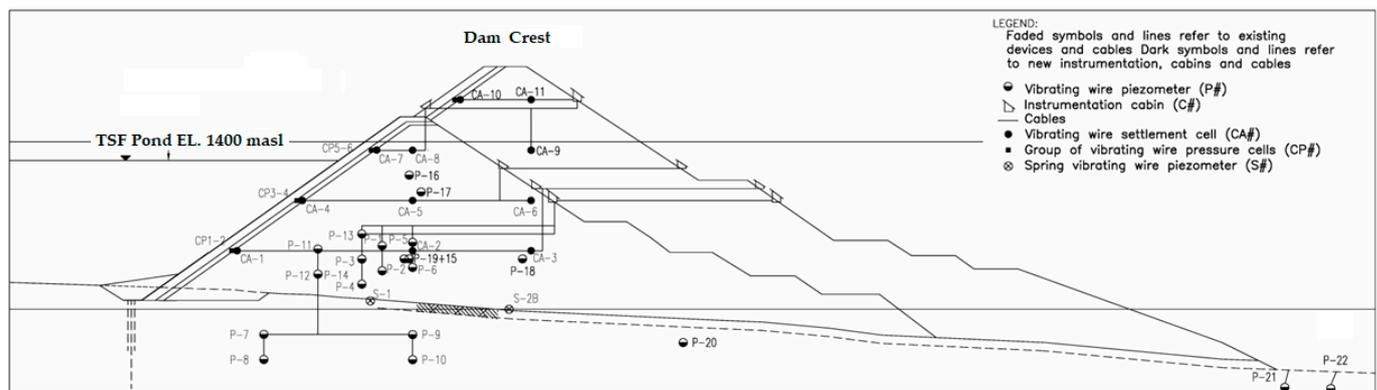
Figure 23. Example of the implementation of an invasive sensor instrumentation system in a mine TSF.
