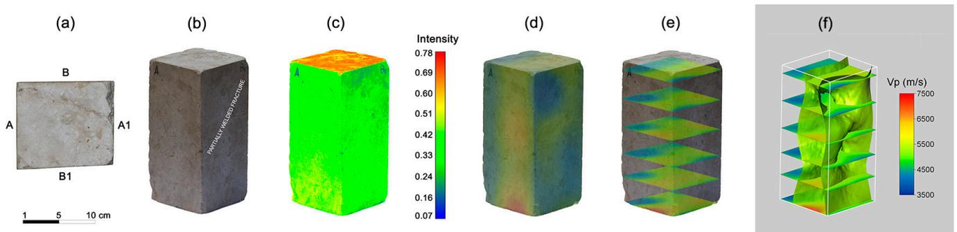
**Figure 12.** Results of the 3D analyses by the integrated approach for the Pietra Forte sample. (a) Localization of the different faces of the sample. (b) 3D HR CRP model texturized with natural colors and represented with an RGB scale. (c) 3D HR CRP model texturized with the intensity of ambient light. (d) 3D ultrasonic tomography incorporated within the 3D HR CRP model. (e) Tomography horizontal slices. (f) Isosurface of 5200 m/s with horizontal slices.
