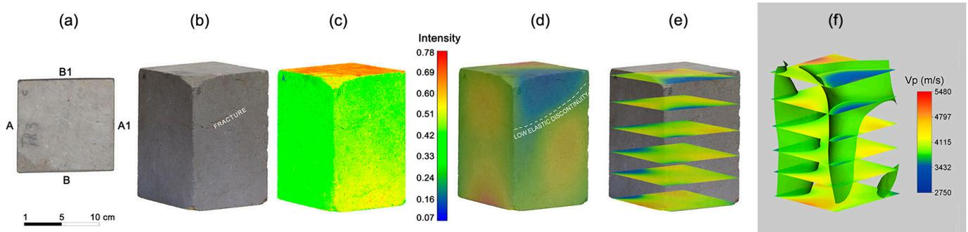
**Figure 10.** Results of the 3D analyses by the integrated approach for the Tramezzario sample. (a) Localization of the different faces of the sample; (b) 3D HR CRP model textured with natural colors and represented in a RGB scale; (c) 3D HR CRP model textured with the intensity of ambient light; (d) 3D ultrasonic tomography incorporated within the 3D HR CRP model; (e) Tomography horizontal slices; (f) Isosurface of 3800 m/s with the horizontal slices.
