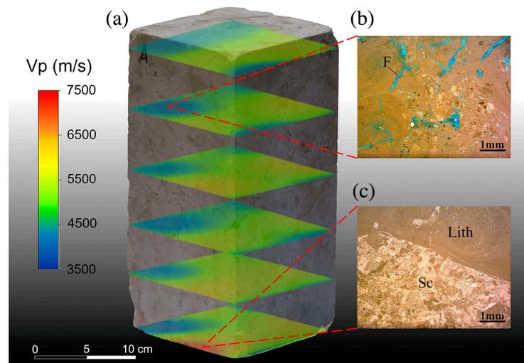
**Figure 13.** Pietra Forte sample: integrated analysis of ultrasonic tomography and thin sections. (a) Tomography horizontal slices incorporated within the 3D HR CRP model. (b) Microscopic features of a porous sector of the sample; OM plane polarized light; thin section treated with blue dye epoxy resin. F (fracture secondary porosity). (c) Microscopic features of a compact sector of the sample; OM cross polarized light. Lith (Lithothamnium algae); Sc (sparry calcite).
