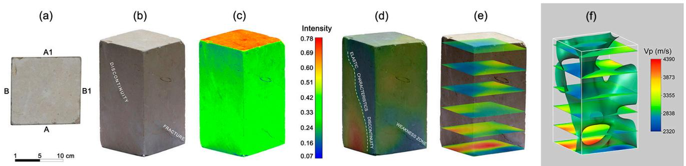
**Figure 8.** Results of the 3D analyses by the integrated approach for the Pietra Cantone sample. (a) Localization of the different faces of the sample. (b) 3D HR CRP model texturized with natural colors and represented with an RGB scale. (c) 3D HR CRP model texturized with the intensity of ambient light. (d) 3D ultrasonic tomography incorporated within the 3D HR CRP model. (e) Tomography horizontal slices. (f) Isosurface of 2800 m/s with horizontal slices.
