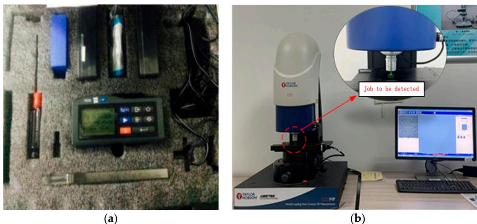
Figure 3. Testing instrument. (a) TR-200 roughness meter; (b) white light interferometer.
