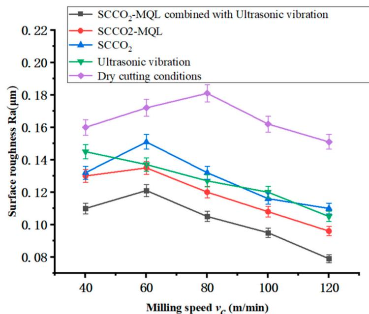
Figure 4. Comparison curve of the influence of process condition on surface roughness with cutting speed.
