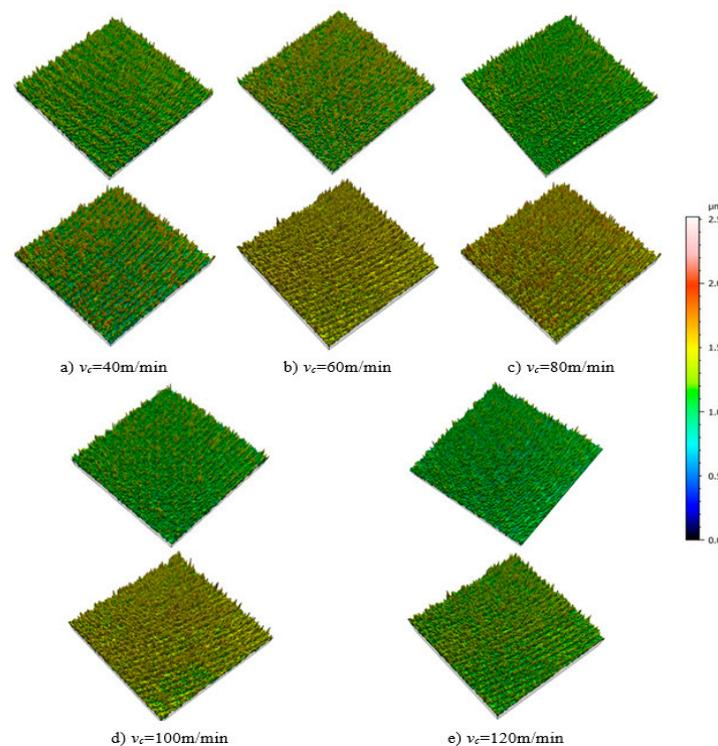
**Figure 9.** Comparison of surface topography of SCCO<sub>2</sub>-MQL combined with ultrasonic vibration (**top**) and dry cutting condition (**bottom**) with cutting speed ( $f = 0.06$  mm/r,  $a_p = 0.6$  mm).
