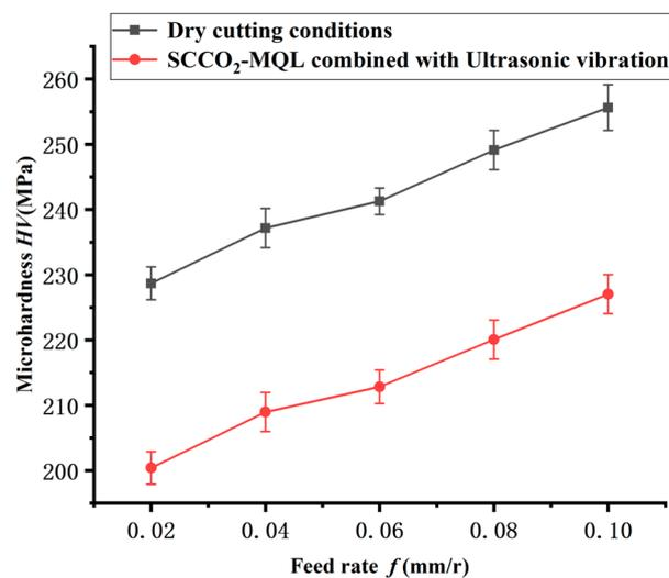
**Figure 15.** The variation curve of microhardness values with feed.
