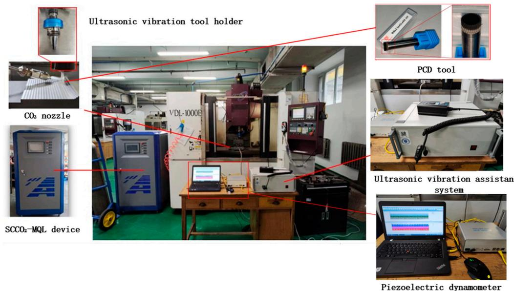
**Figure 1.** VDL-1000 three-axis vertical machining center.
