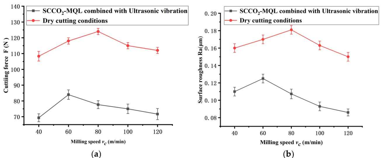
**Figure 6.** Variation in surface roughness with milling speed ( $f = 0.06$  mm/r,  $a_p = 0.6$  mm). (a) Effect of milling speed on cutting force; (b) effect of milling speed on surface roughness.
