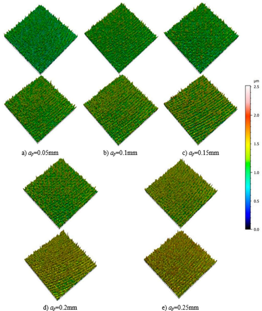
**Figure 11.** Comparison of surface topography of SCCO<sub>2</sub>-MQL combined with ultrasonic vibration (**top**) and dry cutting condition (**bottom**) with cutting depth ( $v_c = 80$  m/min,  $f = 0.06$  mm/r).
