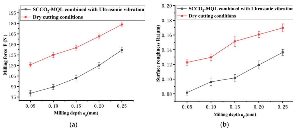
**Figure 8.** Variation in surface roughness with milling depths ( $v_c = 80$  m/min,  $f = 0.06$  mm/r). (a) Effect of milling depths on cutting force; (b) effect of milling depths on surface roughness.
