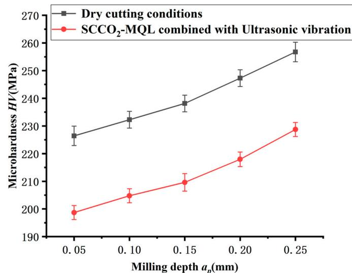
Figure 16. The variation curve of microhardness values with milling depth.
