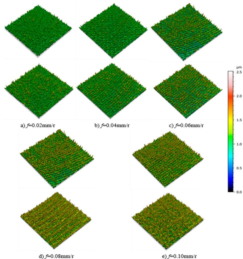
**Figure 10.** Comparison of the surface morphology of SCCO<sub>2</sub>-MQL combined with ultrasonic vibration (**top**) and dry cutting condition (**bottom**) with the change in feed rate ( $v_c = 80$  m/min,  $a_p = 0.6$  mm).
