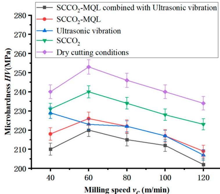
Figure 13. Microhardness curves under different lubrication conditions.
