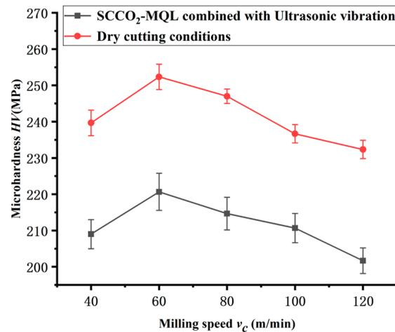
**Figure 14.** The variation curve of microhardness values with milling speed.
