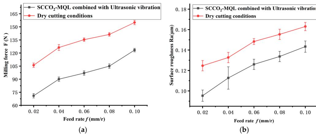
**Figure 7.** Variation in surface roughness with feed rate ( $v_c = 80$  m/min,  $a_p = 0.6$  mm). (a) Effect of feed rate on cutting force; (b) effect of feed rate on surface roughness.
