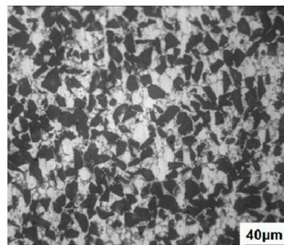
Figure 2. Microstructure of SiCp/Al composites.
