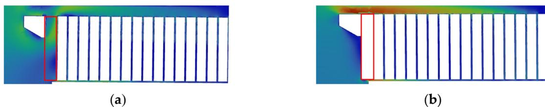
Figure 11. Velocity contours of the air for the effect of insulation between compression plate and laminations: (a) without insulation; (b) with insulation. The red box shows the insulation section.
