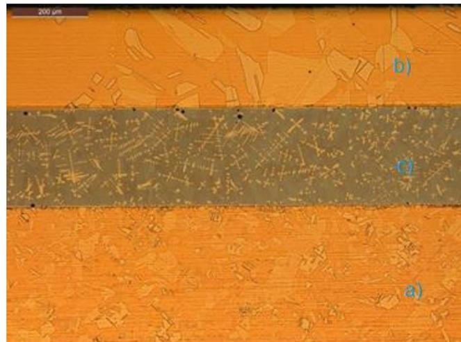
**Figure 20.** Optical microscopy image depicting a longitudinal cross-section of a copper-copper brazing joint. (a) Cu-DHP with averaged grain size 16–60 mm, (b) Cu-DHP with coarse grain size, (c) brazing material.
