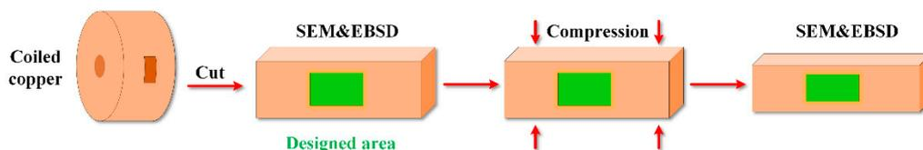
**Figure 1.** Schematic illustrating the quasi in situ deformation and characterization.
