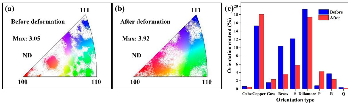
**Figure 5.** Inverse pole figures and orientation contents of a specimen. (a) before compression. (b) after compression. (c) orientation contents change.
