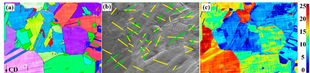
**Figure 11.** Orientation imaging map, SEM map, and the reconstructed SFDR map of the testing region. (a) OIM. (b) SEM map. (c) The reconstructed SFDR map.
