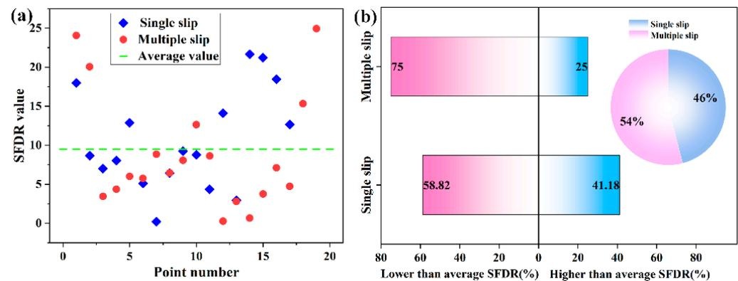
**Figure 10.** SFDR for the extracted grains and its reflection for single and multiple slip system activation.
