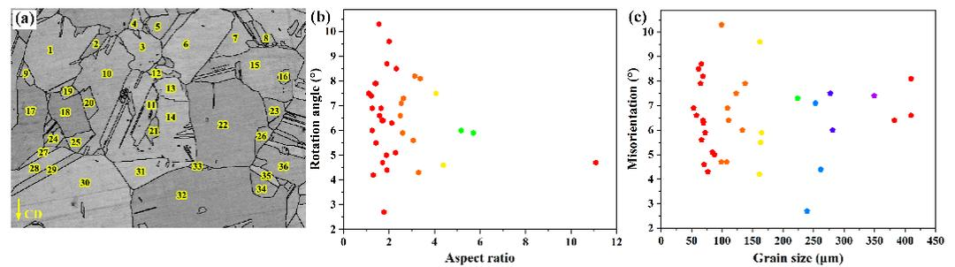
**Figure 6.** Grain rotation and its influencing factors. (a) Numbered grains. (b) Aspect ratio influence on grain rotation. (c) Grain size influence on grain rotation.
