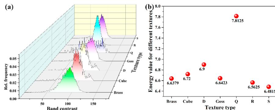
**Figure 8.** Band contrast distribution of the different orientations and the corresponding stored energy values.
