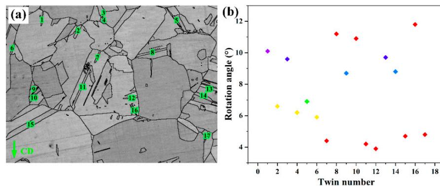
**Figure 7.** Twin rotation during compression. (a) Numbered twins. (b) Rotation degrees for the numbered twins.
