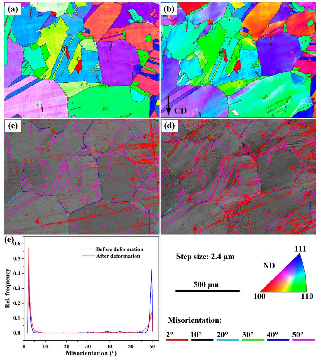
**Figure 4.** EBSD maps of the specimen before and after compression. (a,b) are orientation imaging maps of the testing region. (c,d) are grain boundary maps of the testing region. (e) shows the misorientation evolution during compression.
