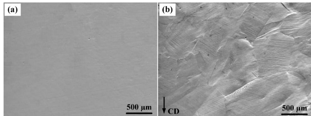
**Figure 3.** SEM maps of specimen: (a) before compression, (b) after compression.
