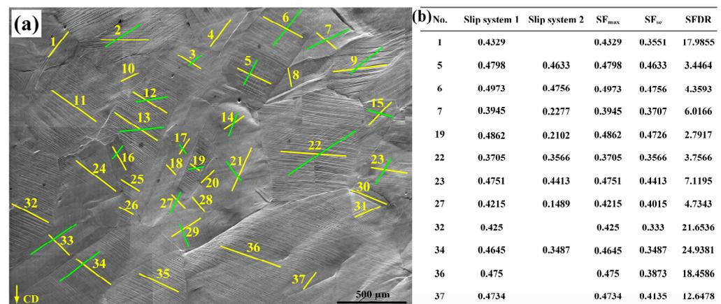
**Figure 9.** Slip trace calibration and the corresponding SFs. (a) Slip trace calibration. (b) SFs of the slip systems.
