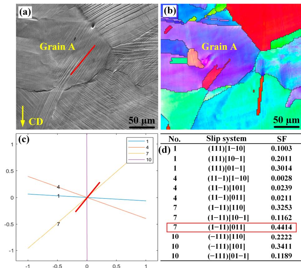
**Figure 2.** Methodology utilized for slip analysis: (a) the occurrence of slip trace (marked using red a line) was tracked by SEM imaging. (b) EBSD OIM was carried out to identify the crystallographic orientation of the slip trace in (a). (c,d) calculation of the four possible traces and SFs for the crystallographic orientation at which a trace was detected and determination of the active slip system. CD here means the compress direction.
