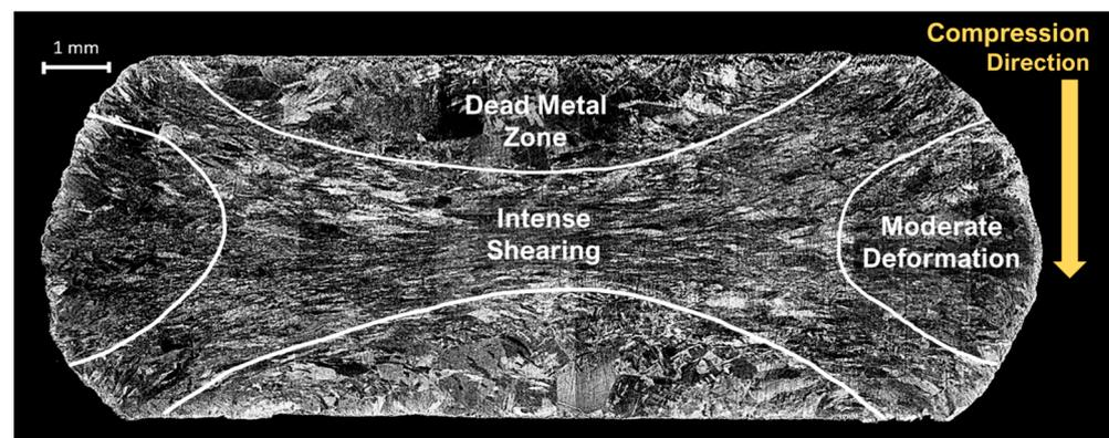
**Figure 5.** Cross-section view of a  $\beta$ -annealed (940 °C/1 h/furnace cool) sample, reheated at 750 °C for 30 min, uniaxially deformed in compression ( $\epsilon = -0.8$ ), and then prepared metallographically to highlight the deformation zones.
