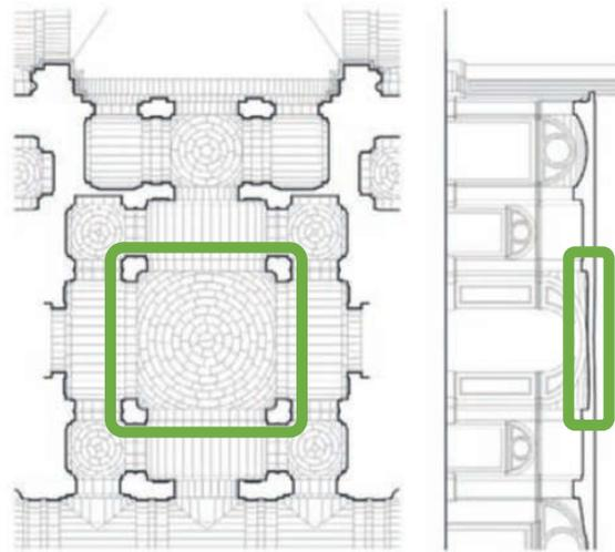
**Figure 7.** Narthex of the Basilica of El Escorial, under choir left: floor plan (left) and section (right), with the flat vault analysed in this article marked in green [7].
