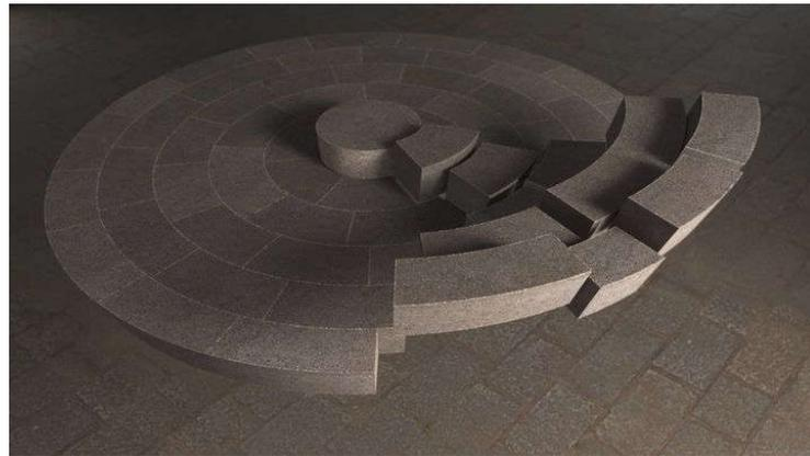
**Figure 14.** Virtual simulation of construction of planar vault voussoirs (graph courtesy by Tele-madrid [14]).
