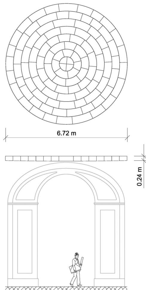
**Figure 11.** Plan with exploded views of voussoirs and section of planar vault (graph by author).
