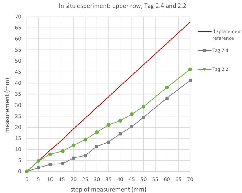
**Figure 45.** In situ experimental test on the 2nd wall: the displacements detected by the upper row Tags 2.4 and 2.2 are compared to the calculated displacements detected by the wired transducer.
