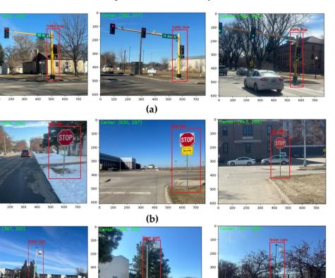
ror for traffic poles, a 4.6 to 5.7 m error for stop signs, and a 5.3 to 6.5 m error for streetlights. These errors serve as indicators of precision and reliability in real-world scenarios.
