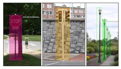
**Figure 2.** Instances of annotated images for training object detection model. Screens are taken from CVAT environment, where bounding boxes are drawn manually.
