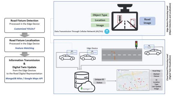
Figure 1. Overview of the proposed road fixture monitoring system.
