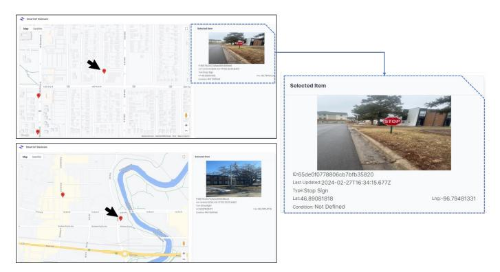
**Figure 7.** Fixture representation on road DT (arrows and dashed boxes were manually added to the screenshots).
