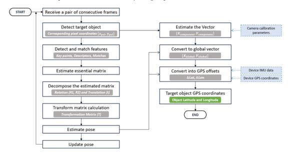
Figure 3. Process of geo-localization of the detected object.
