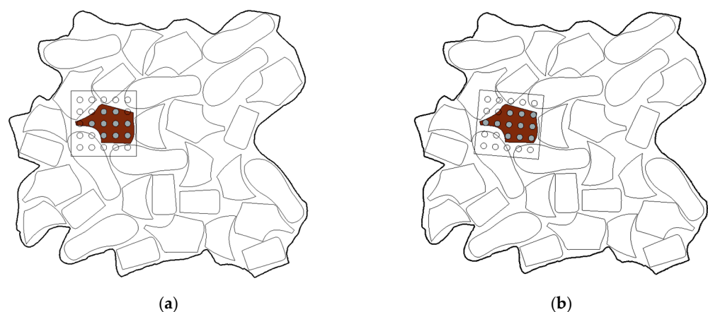
Figure 9. Gripper of a piece with a generic matrix gripper (circles are the vacuum cups and brown piece is the pick piece): (a) Gripping by assigning the position and orientation of the workpiece to the robot end effector: seven gripping points, and (b) Gripping of the workpiece by rotating and moving the tool to maximize the number of gripping points: 11 gripping points.
