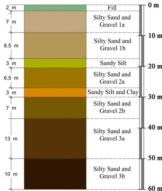
Figure 8. Soil stratigraphy obtained from in situ characterization.
