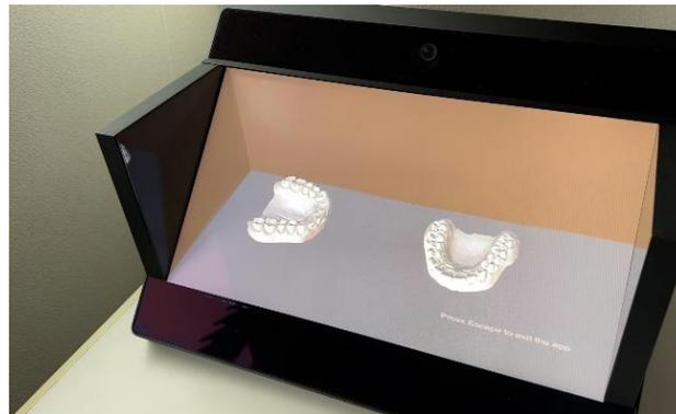
**Figure 5.** 3D-CG model displayed on SRD.
