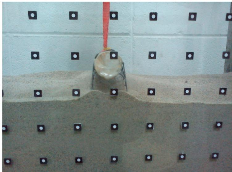
Figure 2. Typical layout of uplift resistance test with single layer geo-grid reinforcement.
