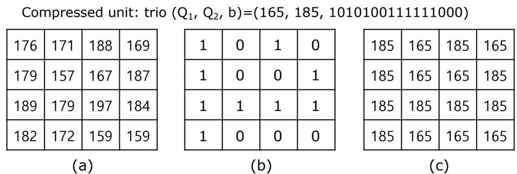
**Figure 1.** An example of AMBTC: (a) an original block; (b) a bitmap block; (c) a reconstruction block.
