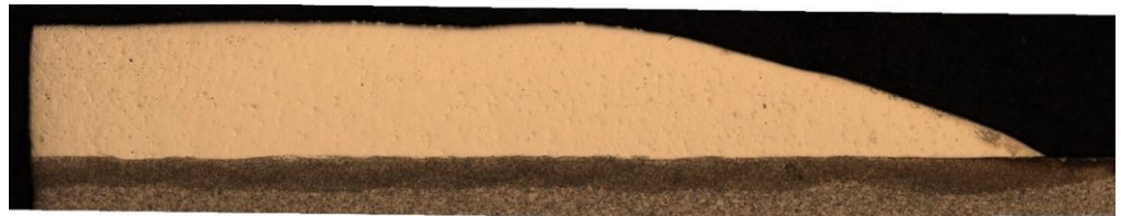
Figure 4. Macrostructure of INCONEL 625 coating cladded on 16Mo3 steel tube, average thickness 2.2 mm ( \times 25 ).
