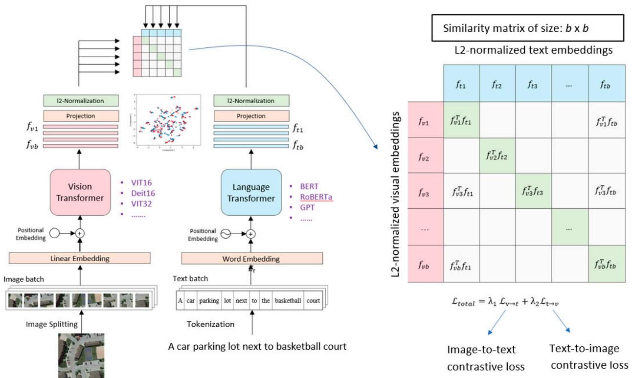
**Figure 2.** Overview of the proposed text–image aligning model. To produce L2-normalized visual  $\{f_{vi}\}_{i=1}^b$  and textual  $\{f_{ti}\}_{i=1}^b$  features, we sample a mini-batch of  $b$  images-text pairings for training the network and feed them to the vision and language transformer encoders. Then, we generate a similarity matrix of size  $b \times b$  by calculating the similarity between all potential visual and textual pairs in the mini-batch.
