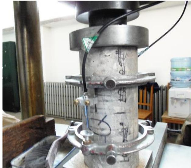
**Figure 5.** Static compressive elastic modulus test.
