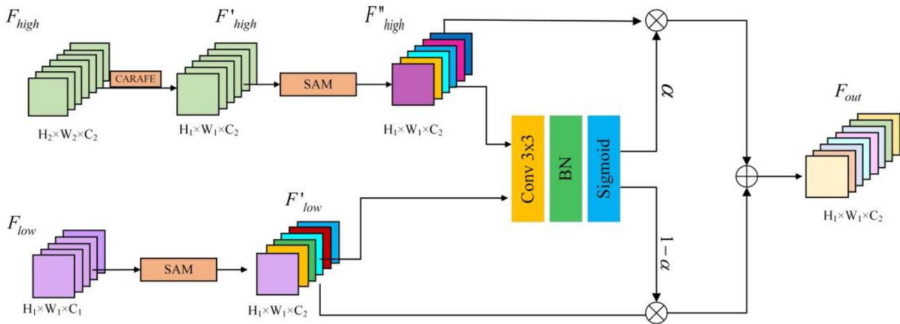
**Figure 4.** The overall architecture of FRAFM. The  $F_{low}, F'_{low}$  represents low feature maps, and the  $F_{high}, F'_{high}, F''_{high}$  represents high feature maps, where  $\alpha, 1 - \alpha \in R^{1 \times H_1 \times W_1}$ .
