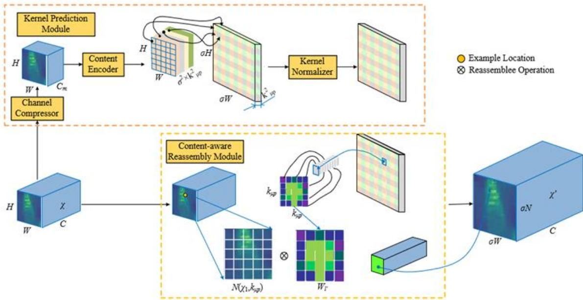
Figure 5. Schematic representation of the CARAFE up-sampling operator structure.
