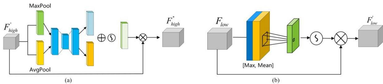
Figure 6. The overall architecture of the CAM and SAM. (a) is CAM that is used for  $F_H$ . (b) is SAM used for  $F_L$ . The  $F_L, F_H$ ; respectively, they represent low feature maps and deep feature maps.
