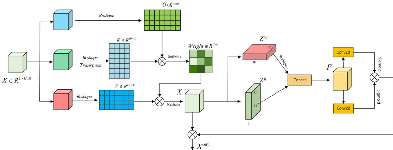
**Figure 7.** CIPAM structure. Each channel feature map is regenerated and then uses horizontal and vertical pooling layers to capture the generated key position information.
