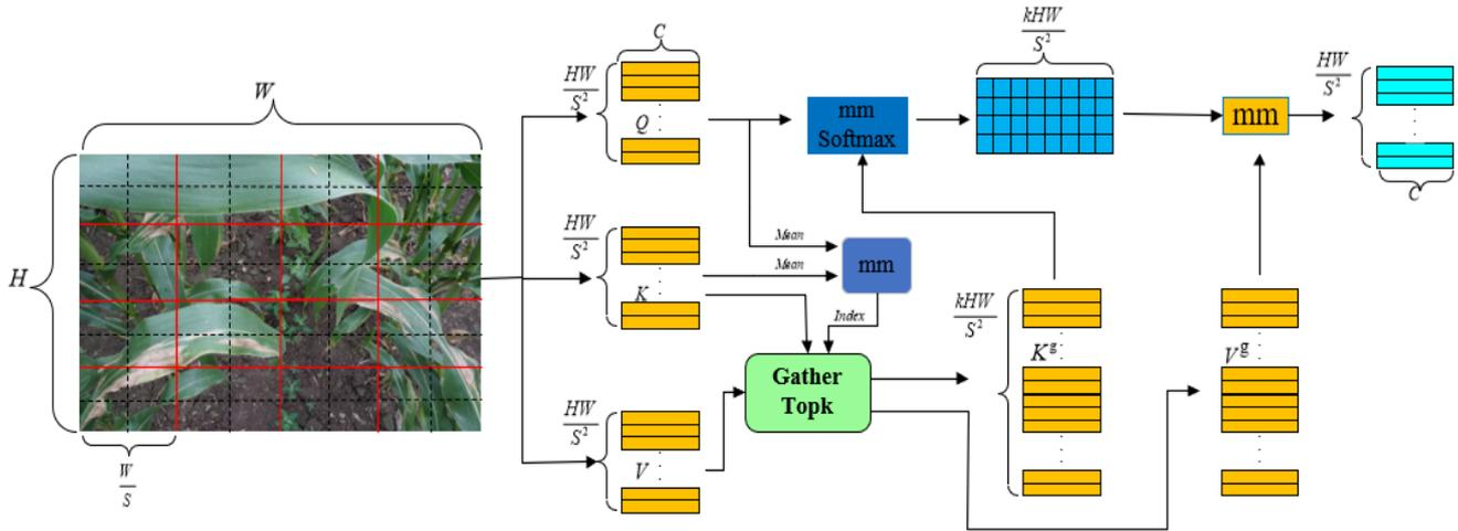
**Figure 3.** The overall architecture of the bi-level transformer with a coarse-grained relationship graph to filter the most relevant  $k$  candidate patches for each patch; then fine-grained token-to-token attention are applied to candidate patches.
