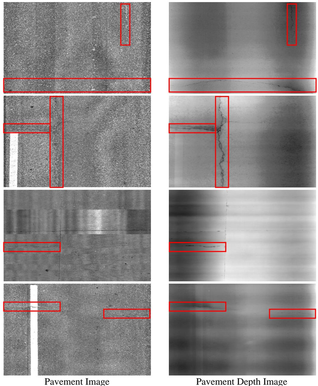
**Figure 1.** Samples of the pavement image data, with the depth image shown simultaneously for clarity considerations (only the left grayscale image is used in the model for applicable fitness considerations). It can be seen that the target shown in the red box (distress) is only a small part of the whole image pixels, reflecting the sparse feature.
