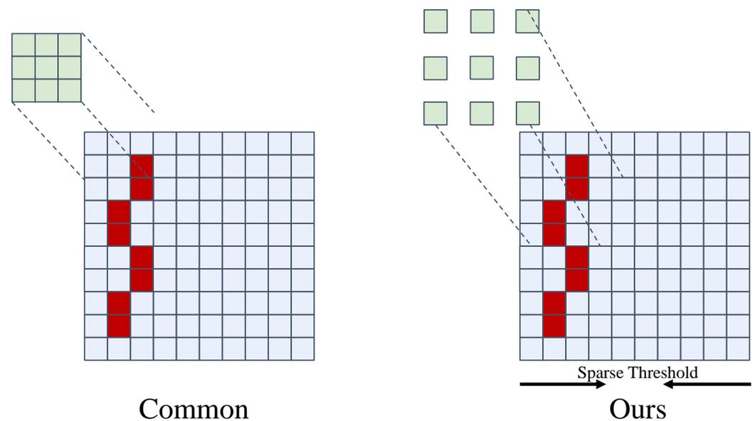
**Figure 3.** The figure demonstrates the difference in feature extraction for pavement distress, where the red box represents the target, the green box represents the convolutional kernel and the blue box represents the background. It can be seen that we have improved the qualitative feature extraction by expanding the receptive field and setting the sparse threshold (0.1).
