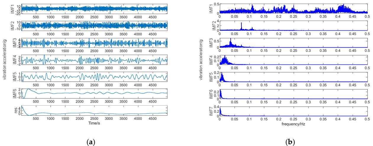
**Figure 4.** Original data and EMD decomposition results of each sequence. (a) Time-domain diagram of the EMD decomposition. (b) Spectrogram of the EMD decomposition.
