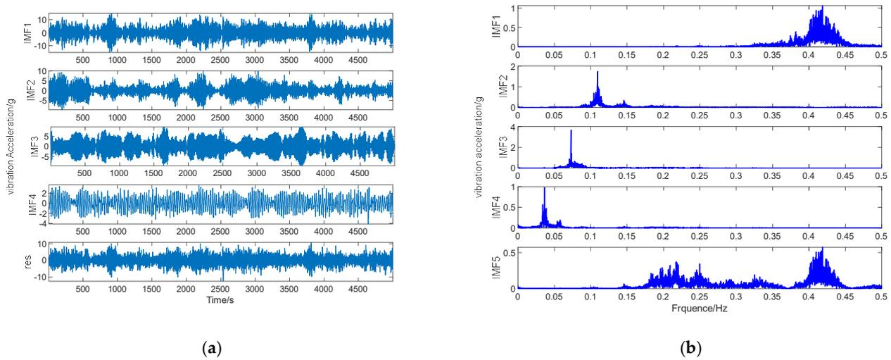
**Figure 3.** Original data and VMD decomposition results of each sequence. (a) Time-domain diagram of the VMD decomposition. (b) Spectrogram of the VMD decomposition.
