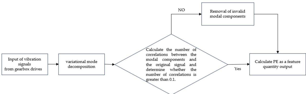
Figure 2. Flow chart of fault feature extraction.
