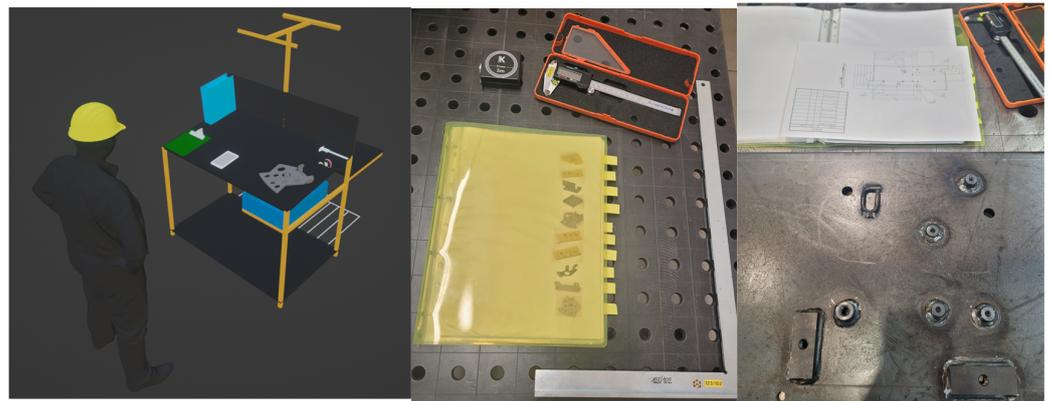
**Figure 5.** Workstation for conventional paper-based inspection.
