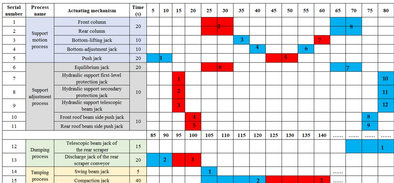
Figure 5. Time sequence of all actions of the cylinders involved in a complete hydraulic support movement-discharge-filling cycle for a single support.
