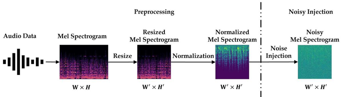
Figure 3. Preprocessing and noise injection of data.
