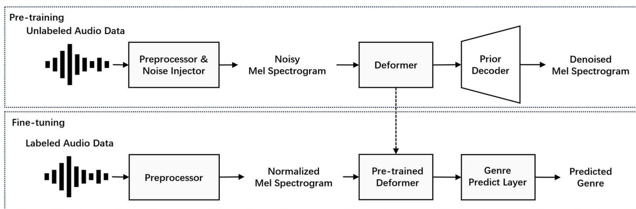
**Figure 1.** Overview of the method: pre-training and fine-tuning stages.
