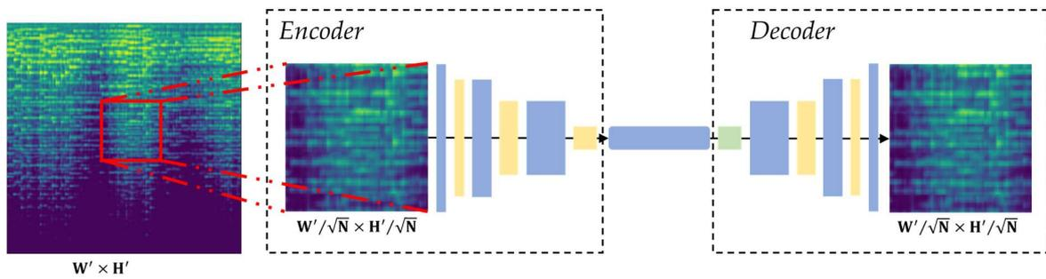
Figure 4. Structure of the autoencoder.
