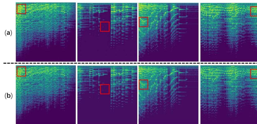
**Figure 8.** Output of the decoder. (a) Reconstructed Mel spectrograms and (b) original Mel spectrograms. The red boxes indicate subtle differences between (a,b).
