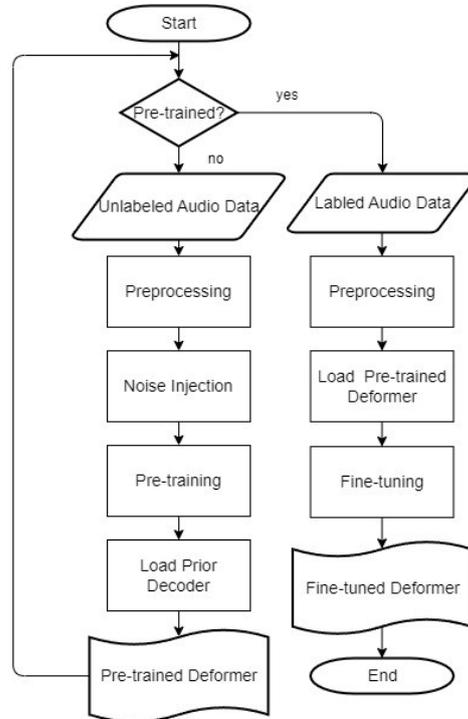
Figure 2. Flowchart of pre-training and fine-tuning under the proposed method.
