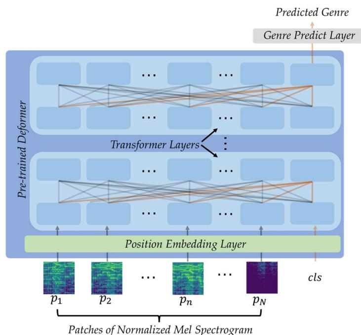
Figure 6. Fine-tuning stage of Deformer.
