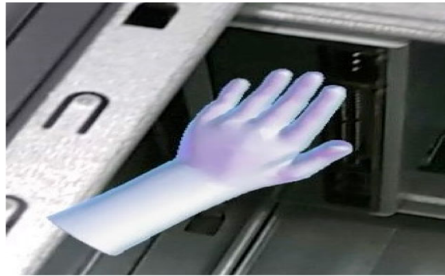
Figure 10. A virtual hand shows that a push on the DVD drive is needed to remove it from computer case.
