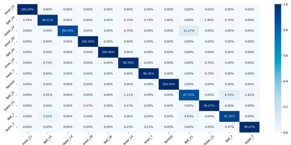
Figure 8. A confusion matrix of vector-CFNN for various sizes of damage diameter classification.
