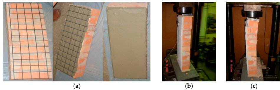
**Figure 4.** Masonry segment made of ceramic bricks, cross-section  $12 \times 25$  cm, reinforced with a steel mesh: (a) from preparation; (b) under load; (c) destruction.
