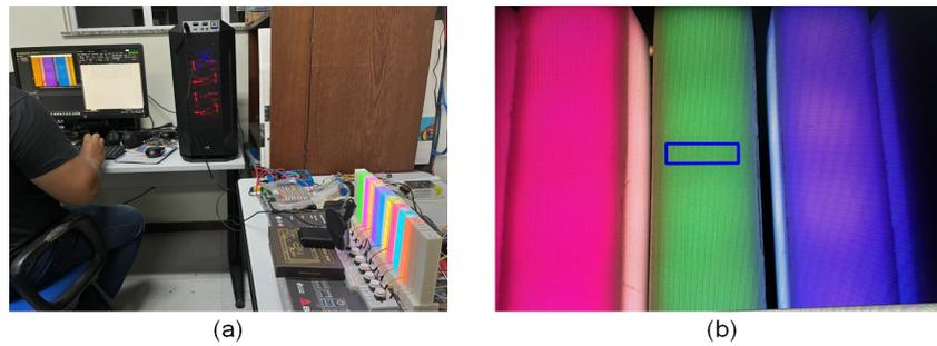
**Figure 15.** Setting the LED strip brightness setting. (a) Configuration by the facilitator of the colors in the physical bars (b) Image of the bar to measure luminance and color. The blue rectangle indicates the area of the bar that the image processing algorithms are applied.
