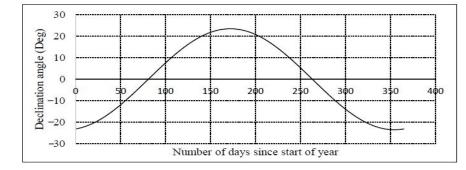
Figure 3. Variation of the declination angle with n days over the year.
