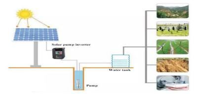
Figure 1. Typical photovoltaic solar water pumping station.
