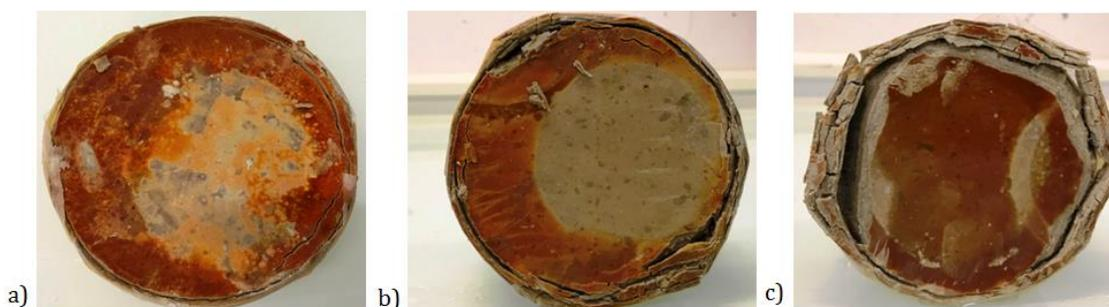
**Figure 5.** Degradation of cement paste due to ESA: (a) after 12 weeks; (b) after 20 weeks; (c) after 24 weeks.
