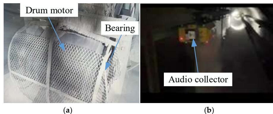
**Figure 9.** Drum motor for the coal mine transportation (the collected data on the bearings of the underground drum motor was used for the cross-working condition fault diagnosis). (a) Drum motor; (b) Audio acquisition device.
