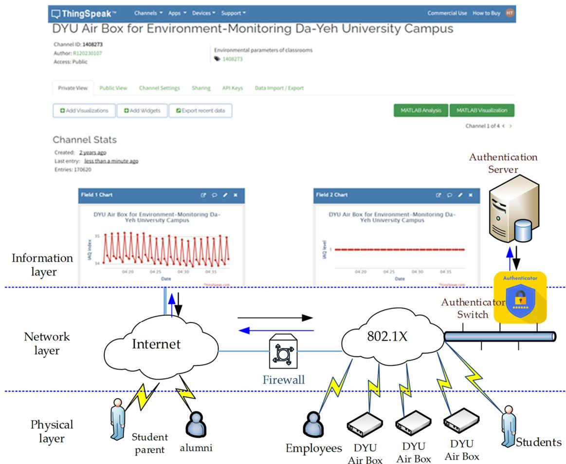
**Figure 1.** Schematic of wireless multi-sensor EMIoT system on Da-Yeh University campus.
