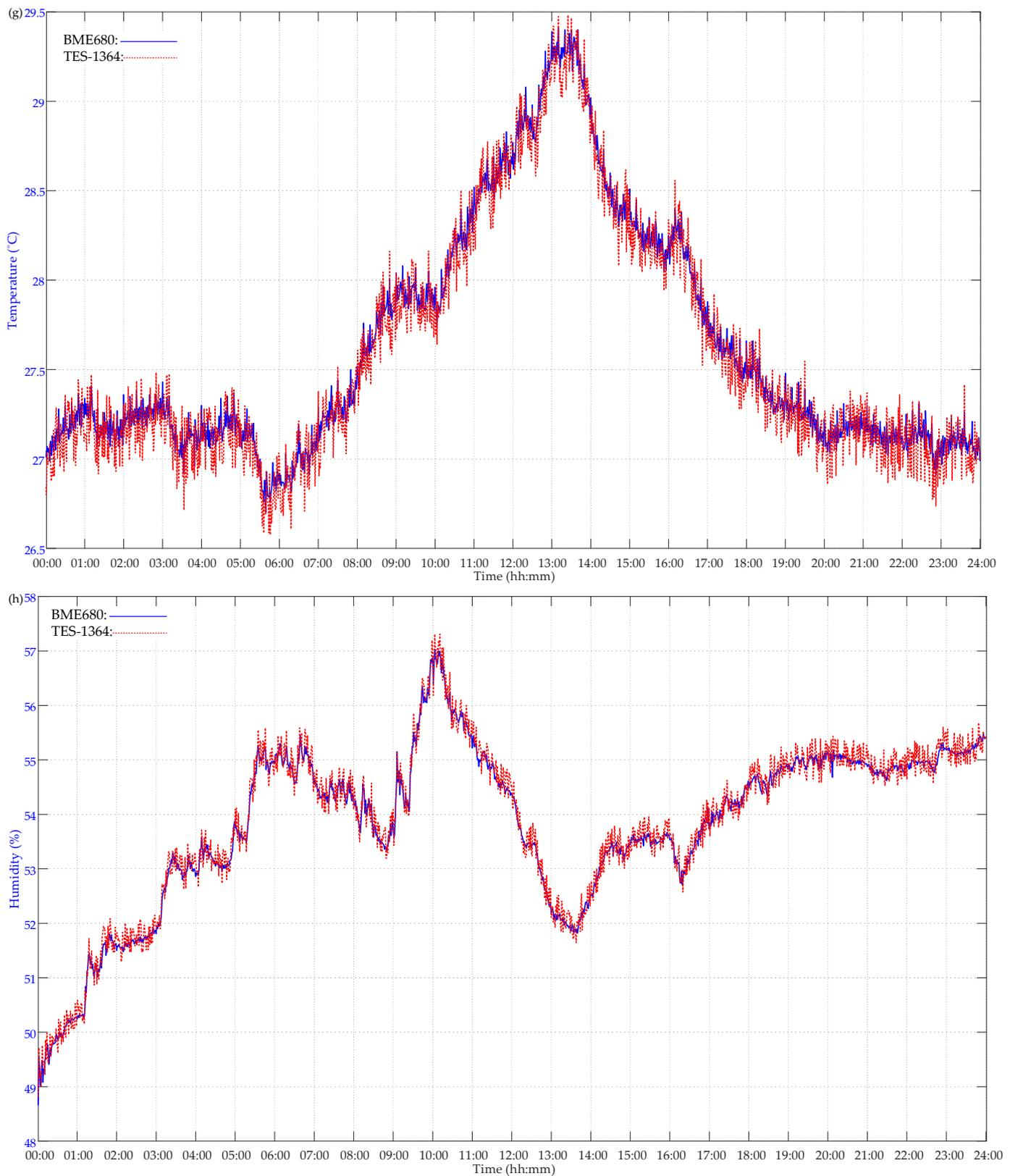
**Figure 7.** The 24 h in situ measurement results of DYU Air Box for environmental monitoring of H708 classroom at Da-Yeh University: (a) IAQ index; (b) IAQ level; (c) PM<sub>1,0</sub> concentration; (d) PM<sub>2,5</sub> concentration; (e) CO<sub>2</sub> concentration; (f) brightness; (g) temperature; (h) humidity.
