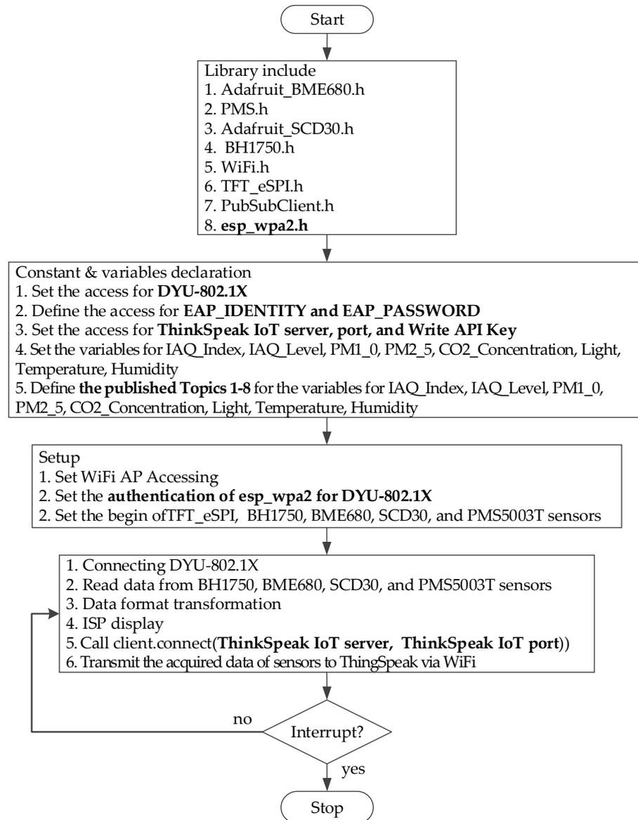
Figure 4. The flowchart of the proposed wireless DYU Air Box.
