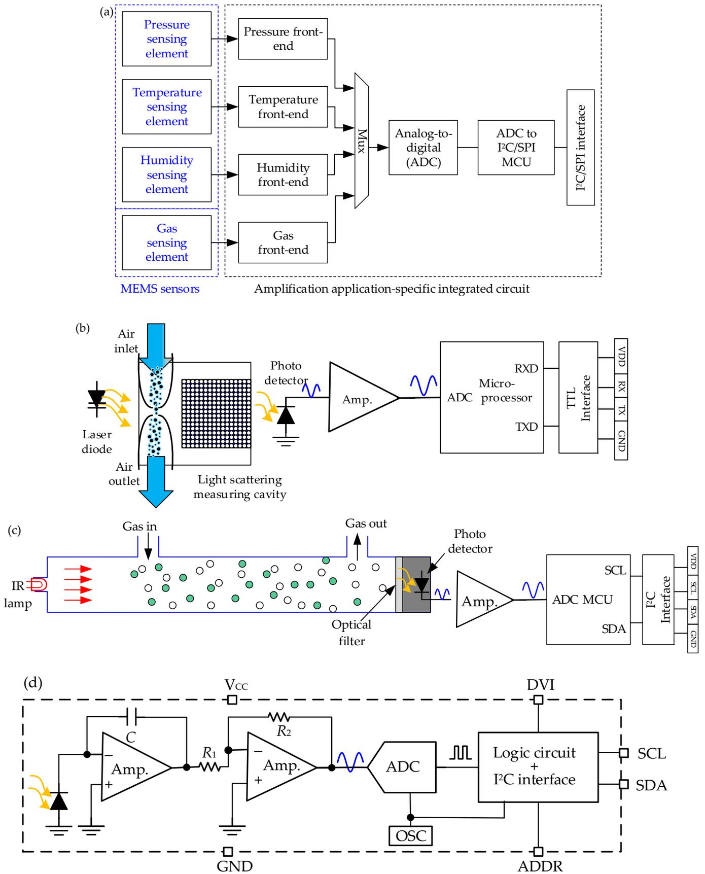
**Figure 3.** Schematics of heterogeneous sensors: (a) BME680 air quality sensor; (b) PMS7003T dust sensor; (c) SCD30 CO<sub>2</sub> gas sensor; (d) BH1750 light sensor.
