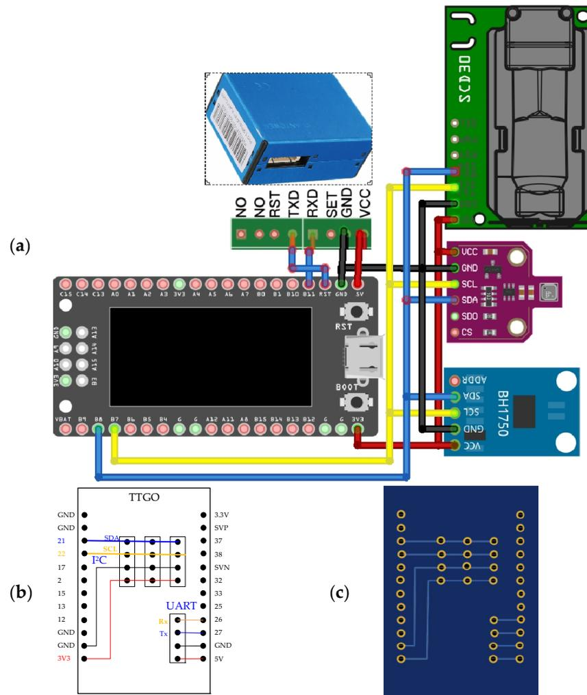
**Figure 2.** Schematics of wireless DYU Air Box with heterogeneous and multi-sensor module: (a) Wiring connection; (b) sensor shield; (c) PCB layout.
