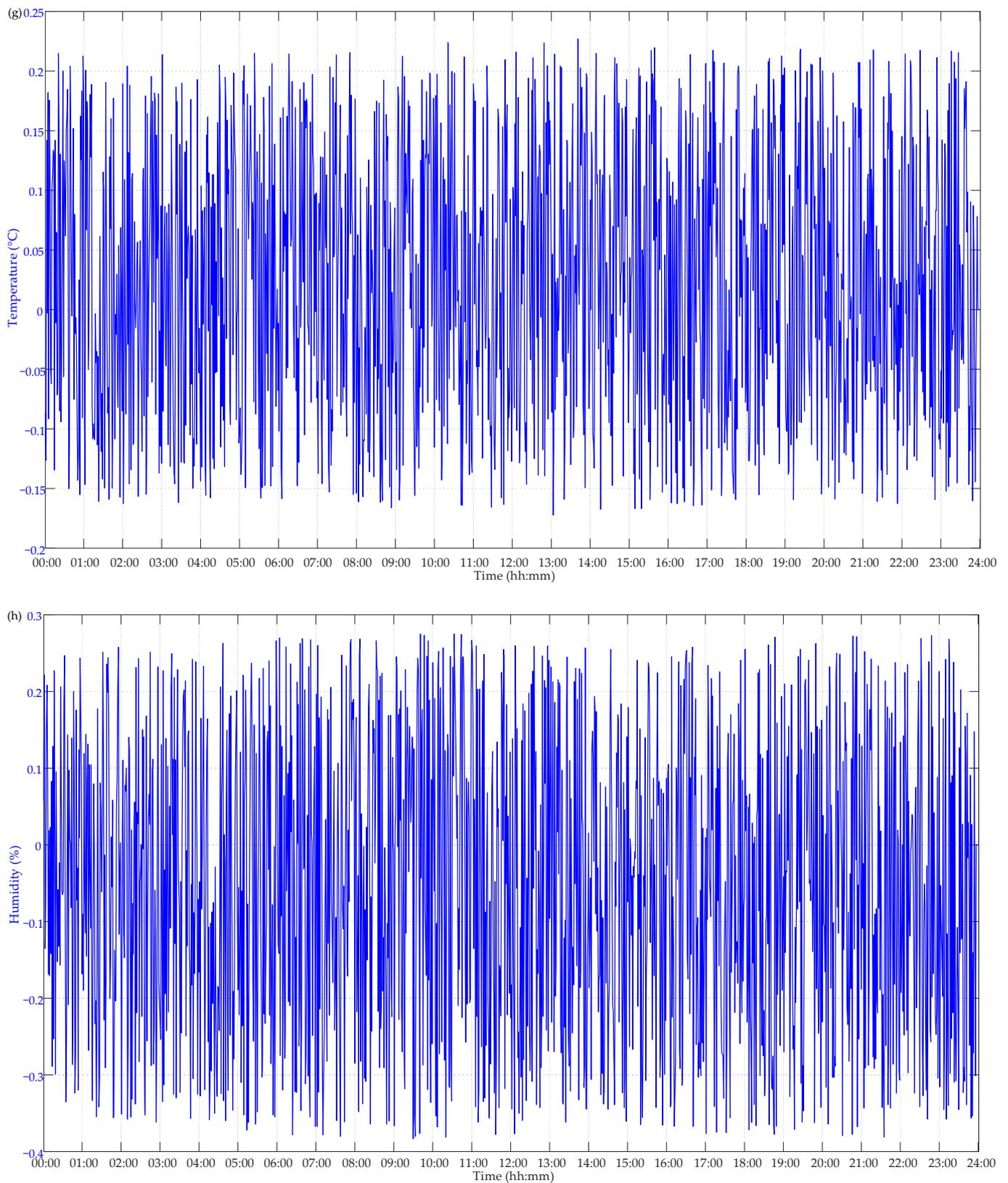
**Figure 8.** Difference analysis of 24 h in situ measurement results for DYU Air Box compared with corresponding measurement instruments: (a) IAQ index; (b) IAQ level; (c) PM<sub>1.0</sub> concentration; (d) PM<sub>2.5</sub> concentration; (e) CO<sub>2</sub> concentration; (f) brightness; (g) temperature; (h) humidity.
