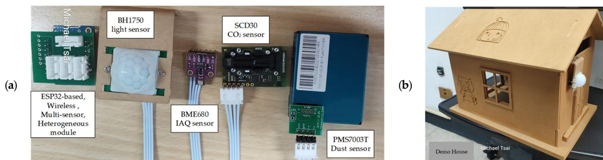
**Figure 5.** Photographs of the proposed wireless heterogeneous multi-sensor module: (a) TTGO ESP32 Wi-Fi module, BH1750 light sensor, BME680 AQI sensor, SCD30  $CO_2$  sensor, and PMS7003T dust sensor; (b) demo DYU Air Box for environmental monitoring of classroom.
