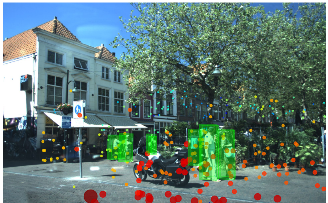
Figure 1. The detection of vulnerable road users (VRU) from 4D radar data (colored dots) is particularly challenging due to the sparsity of radar sensor data, especially for small objects. With our SRFF, we present a method that specifically targets the detection (green boxes) of these objects.
