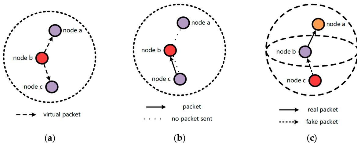
**Figure 2.** Attack model: (a) DDoS attack; (b) selective forwarding attack; (c) data pollution attack.
