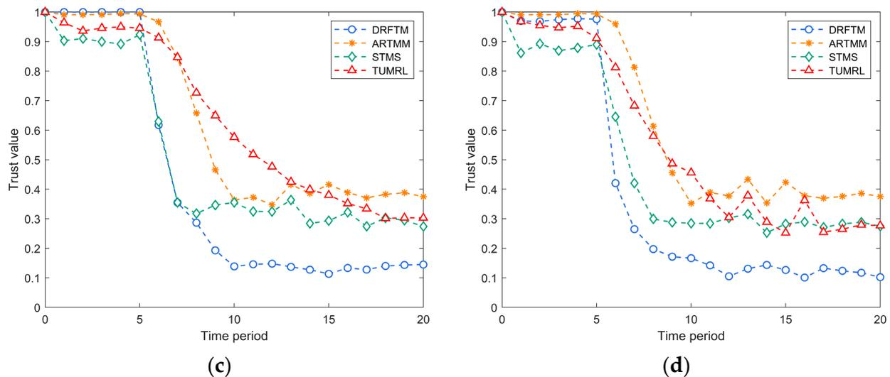
**Figure 9.** Comparison of performance in single-mode attacks: (a) DDoS attack; (b) selective forwarding attack; (c) data pollution attack; (d) on-off attack.
