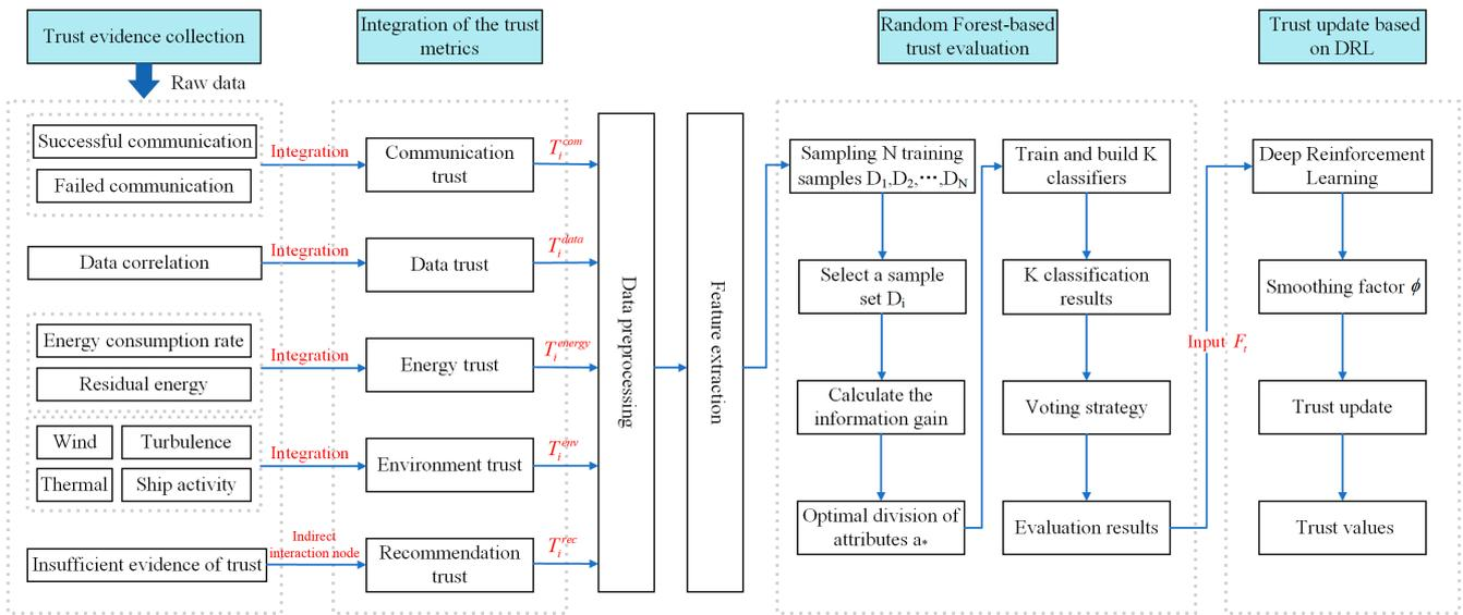
Figure 3. DRFTM architecture diagram.
