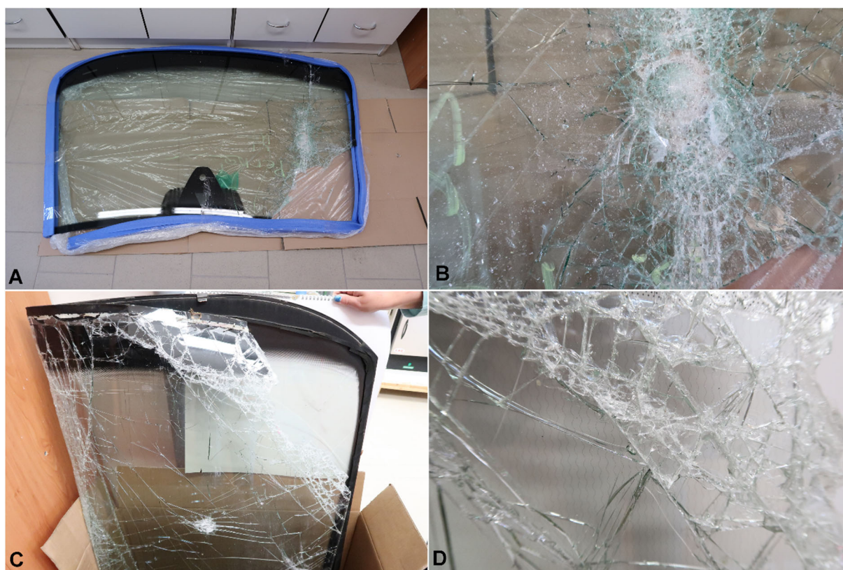
Figure S1. Automotive glass waste used (A and B – general and detailed view on windscreen with protective film, C and D – general and detailed view on windscreen with protective film and heat elements)
