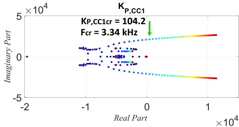
Figure 7. Eigenvalue trace of current controller’s proportional gain variation  $K_{P,CC1}$ , which varied from 0.1 (deep blue) to 10 (deep red) times  $K_{P,CC0}$ . Green arrow means instability point.
