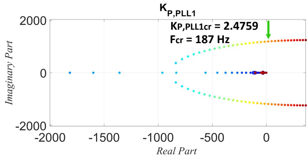
**Figure 8.** Eigenvalue trace of PLL’s proportional gain variation  $K_{P,PLL1}$ , which varied from 0.1 (deep blue) to 20 (deep red) times  $K_{P,PLL0}$ . Green arrow means instability point.
