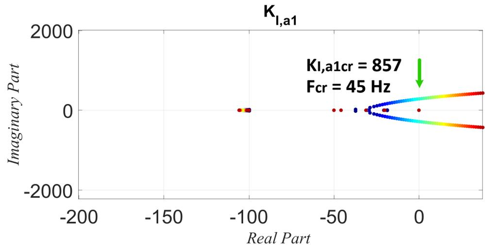
**Figure 9.** Eigenvalue trace of AVC’s integral gain variation  $K_{I,a1}$ , which varied from 0.1 (deep blue) to 200 (deep red) times  $K_{I,a0}$ . Green arrow means instability point.
