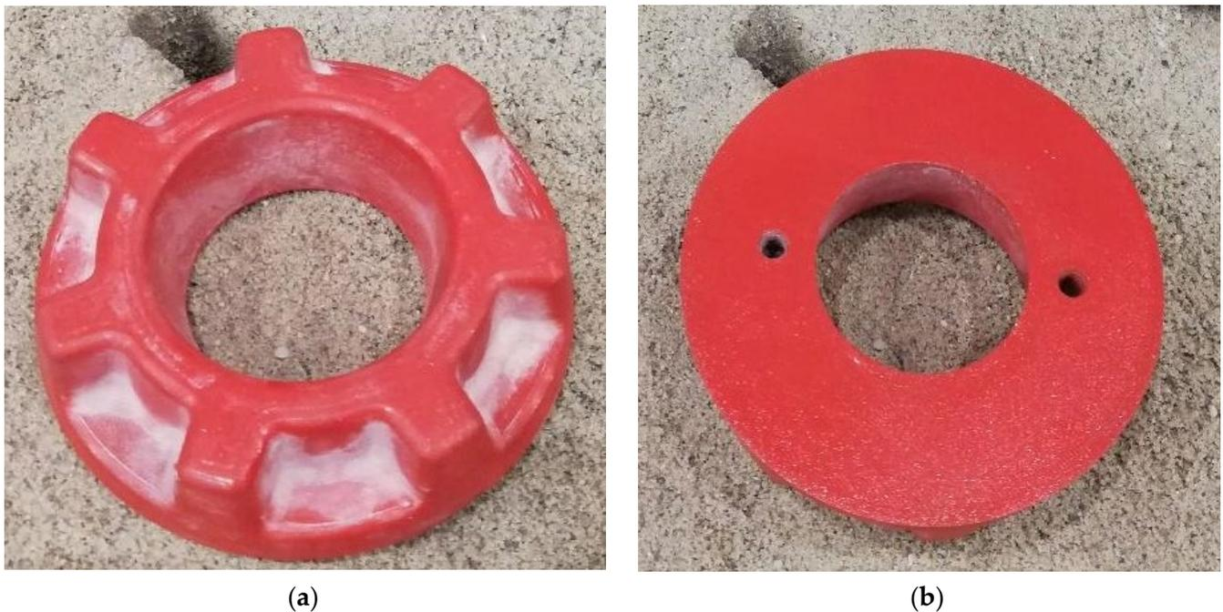
**Figure 4.** Model used to make the cast: (a) top view; (b) bottom view.
