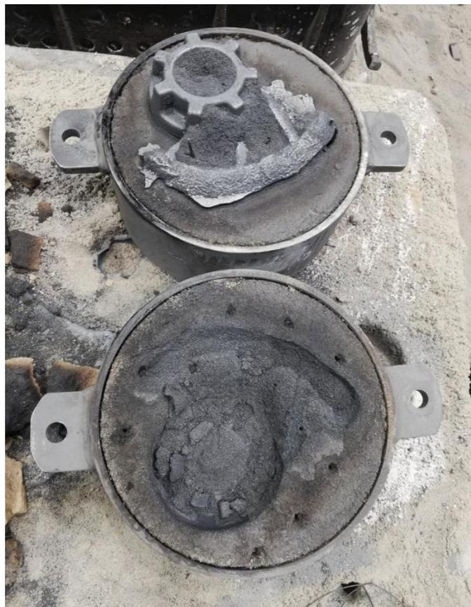
**Figure 9.** View of the casting mould after opening but before knocking out.
