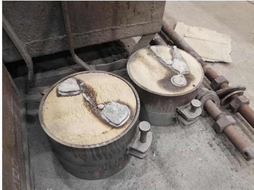
**Figure 8.** View of the casting moulds after casting.
